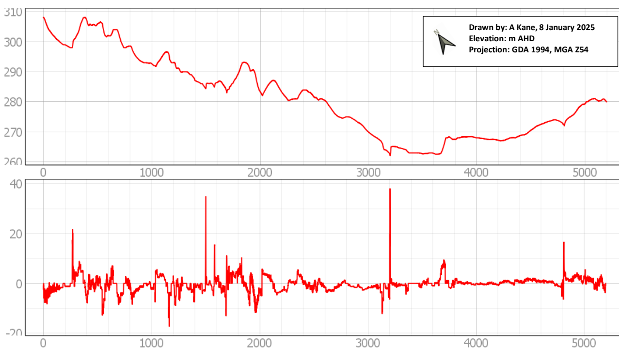
Figure 8-10: Cross-sections, Iron Peak 'Southern' haul road option (m AHD) and slope (degrees)
