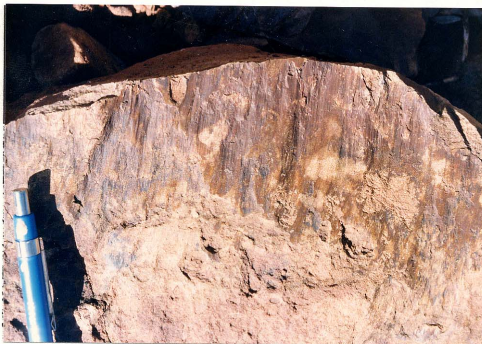
FIGURE 11. CLOSE-UP OF SLICKENSIDES IN SANDSTONE FLOAT, SAMPLE STATION 220.
