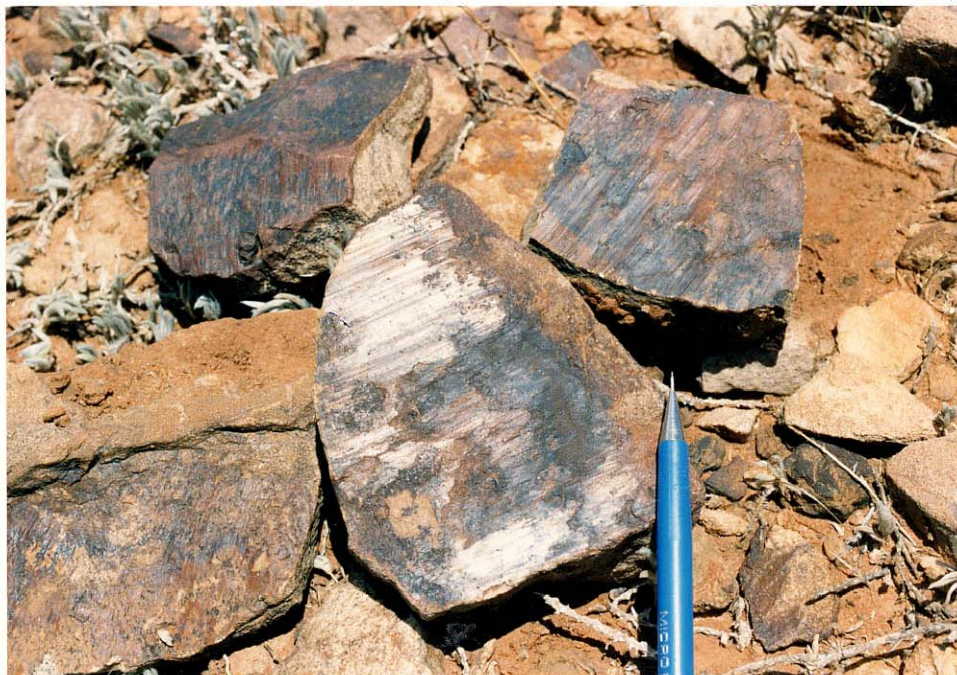
FIGURE 10. SLICKENSIDES IN SANDSTONE FLOAT, SAMPLE STATION 220.
