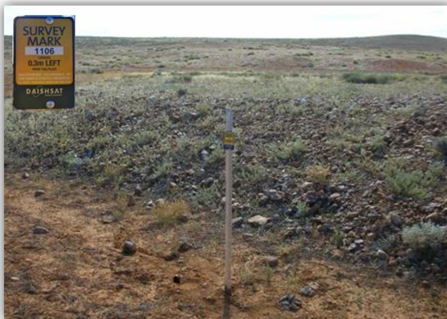
Photo 4 – Base 1106 used for the survey
