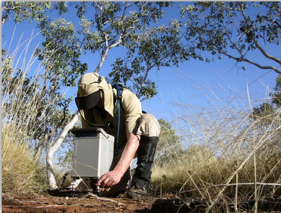
Photo 7 – A Surveyor levelling a Scintrex CG5 gravity meter
