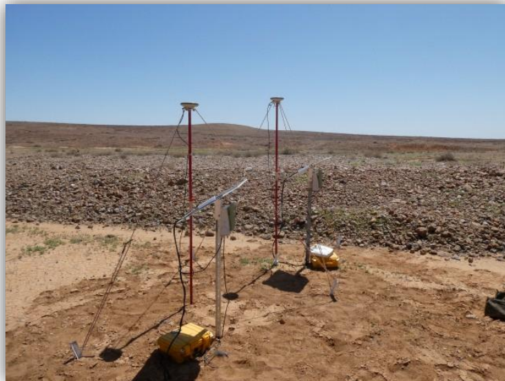
Photo 5 – A Leica GX1230 GNSS receiver set up over base 1106 with a redundant base set up nearby
