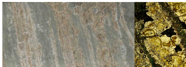
(b) Banded garnet–pyroxene–amphibole–sulfide skarn. Drillhole GHDD01, 932.3 m. Inset: Photomicrograph of drill core sample showing garnet (zoned brown to pale yellow) bands and interstices of amphibole (dark green) and sulfide (mostly black; chalcopyrite, sphalerite, galena). (Photo 416630, 416631)
