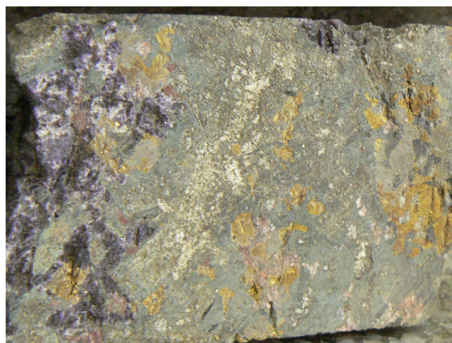
(f) Coarse-grained amphibole–pyroxene–sulfide–fluorite(–gold) skarn. Dull green amphibole, lustrous yellow chalcopyrite, purple fluorite. Drillhole GHDD01, 952 m. (Photo 416635)
