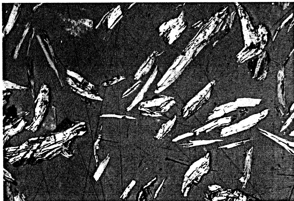
FIG. 7: Sample B, -425\ \mu\text{m} + 150\ \mu\text{m} , <2.4\ \text{sp.gr.} Graphite flakes.
