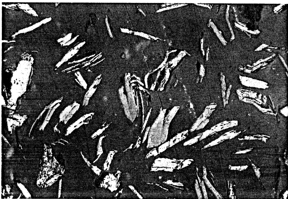
FIG. 8: Sample B, -150\ \mu\text{m} + 75\ \mu\text{m} , <2.4\ \text{sp.gr.} Graphite flakes.
