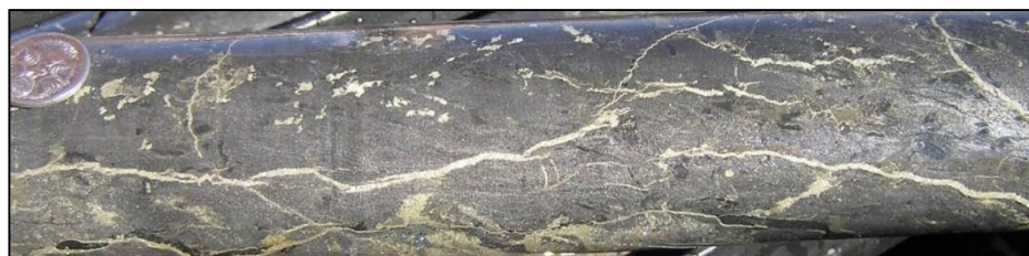
Figure 17: Graphitic schist containing disseminated pyrite and irregular pyrite veinlets at 324.1m, DD16TUR014
