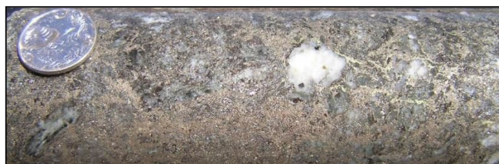
Figure 46: Pyrrhotite-matrix breccia with chalcopyrite-rich trails on right (downhole) of prominent quartz clast, at 227.7m in DD16JUP004. Downhole to the right
