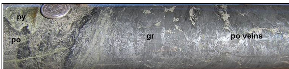
Figure 26: Pyrrhotite-matrix breccia (left) and irregular pyrrhotite veinlets within graphitic schist at 234.2m, DD16TUR016
