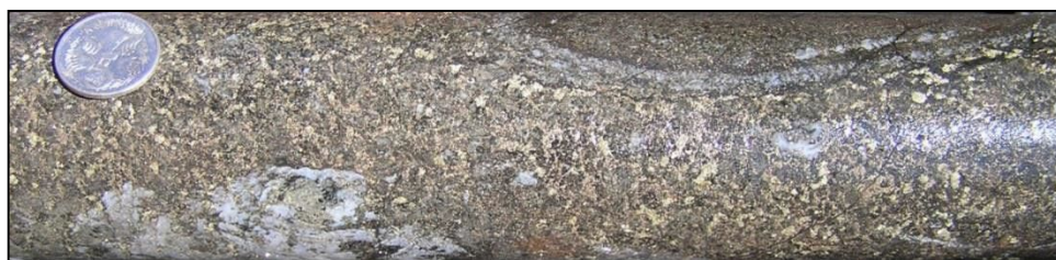
Figure 50: Pyrrhotite- and pyrite-matrix breccia at 294.7m, DD16JUP005
