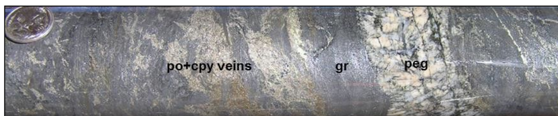
Figure 28: Irregular pyrrhotite + chalcopyrite veinlets within graphitic schist at 247.2m, DD16TUR016
