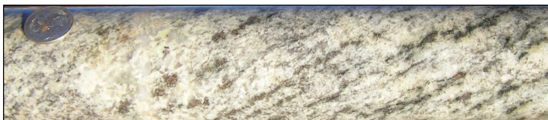
Figure 54: Garnetiferous leucogneiss at 358.5m, DD16JUP005
