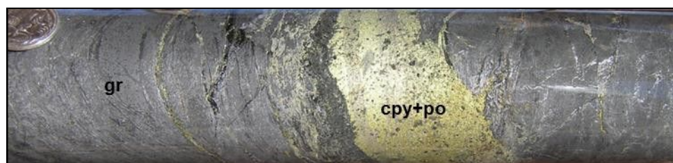
Figure 27: Vein, rich in chalcopyrite and pyrrhotite, within graphitic schist at 246.3m, DD16TUR016
