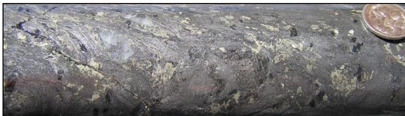
Figure 14: Graphitic and pyritic schist at 253.0m, DD16TUR014
