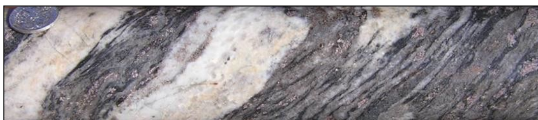
Figure 53: Quartz +feldspar +biotite +garnet paragneiss at 329.6m, DD16JUP005
