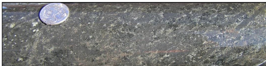
Figure 51: Compositionally banded and foliated ?pyroxenite at 301.0m, DD16JUP005
