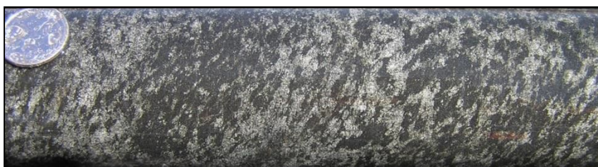
Figure 44: Weakly compositionally banded and strongly foliated (?) pyroxenite at 211.9m, DD16JUP004
