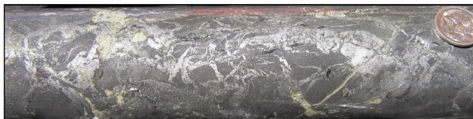
Figure 15: Graphitic schist containing irregular veins of coarser graphite at 260.5m, DD16TUR014
