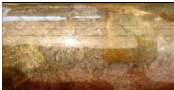
Figure 40: Vein of massive very coarse-grained pyrrhotite and diopside at ~57.5m in hole DD11JUP002 at the Jupiter Prospect.
