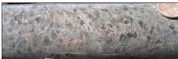
Figure 13: Calcsilicate containing hornblende, diopside and phlogopite at 245.0m, DD16TUR014
