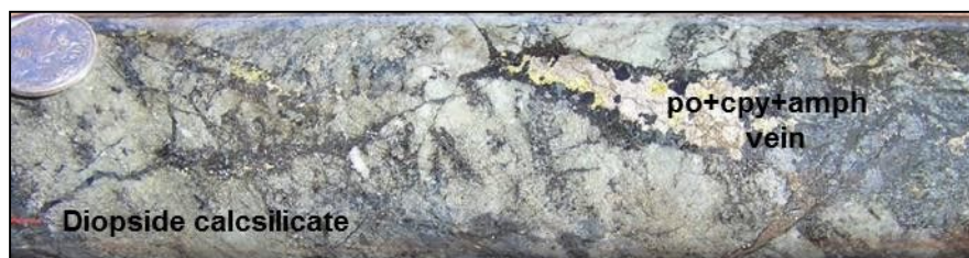
Figure 30: Pyrrhotite +chalcopyrite +amphibole vein within diopside-bearing calcsilicate at 263.6m, DD16TUR016
