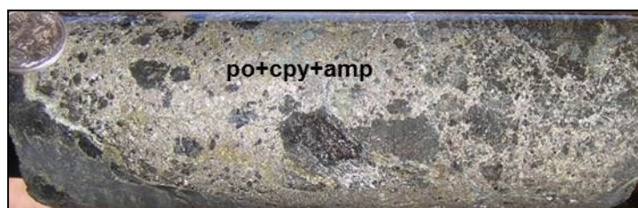
Figure 25: Breccia at 231.5m, DD16TUR016, with matrix consisting predominantly of pyrrhotite, chalcopyrite and hornblende
