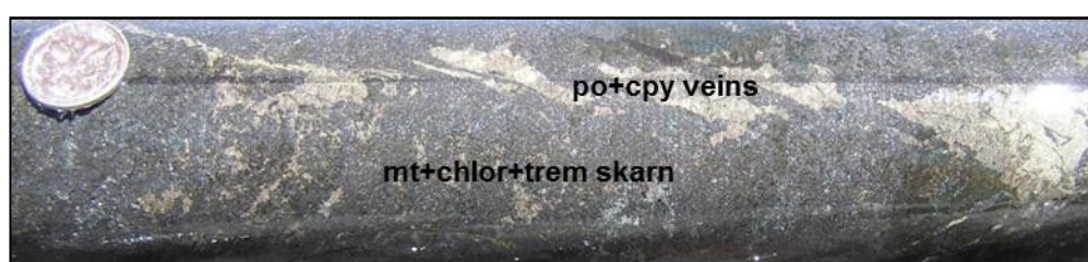
Figure 32: Extensional pyrrhotite + chalcopyrite veins within skarn assemblage of magnetite, chlorite and tremolite at 335.4m, DD16TUR016
