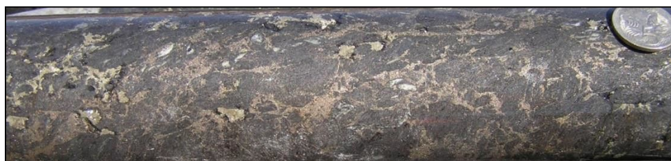
Figure 19: Irregular, semi-continuous pyrrhotite veins and disseminated pyrite within graphitic schist at 350.4m, DD16TUR014
