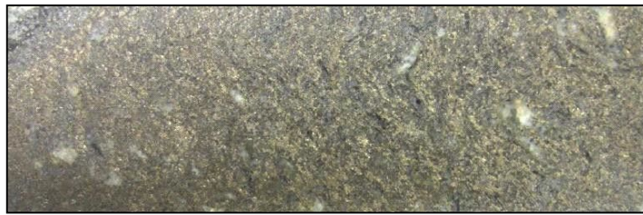
Figure 56: Pyrrhotite-matrix breccia at 226.0–226.18m in DD16JUP004 with measured conductivity of 2,700 S/m (Petrophysics ID 17TR0022)
