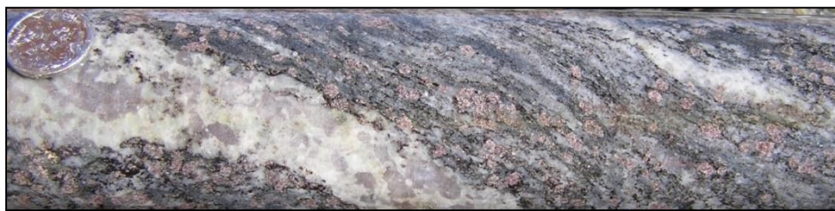
Figure 42: Strongly-foliated garnetiferous, quartz +feldspar +biotite gneiss at 122.4m, DD16JUP004
