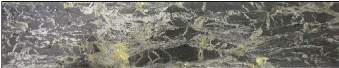
Figure 57: Two-tone graphitic schist with pyrite and pyrrhotite aggregates and veins, 260.0–260.25m in DD16TUR014, with measured conductivity of 810 S/m (Petrophysics ID 17TR0003)
