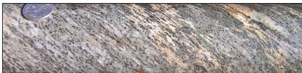
Figure 52: Mylonitised quartz +feldspar +biotite gneiss and hornblende-bearing gneiss at 319.5m, DD16JUP005
