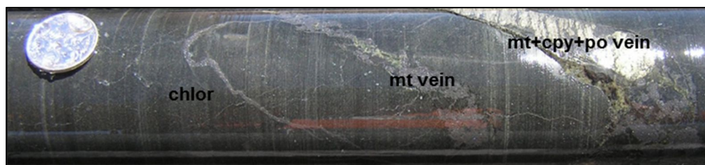
Figure 33: Vein of magnetite + chalcopyrite +pyrrhotite within chlorite-rich skarn at 336.7m, DD16TUR016
