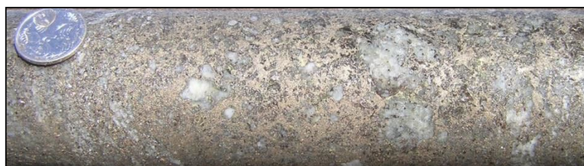
Figure 45: Pyrrhotite-matrix breccia at 225.6m, DD16JUP004
