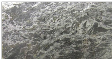
Figure 59: Two-tone graphitic and pyritic schist at 293.6–293.69 in DD10TUR008 with measured conductivity of 500 S/m (Petrophysics ID 17TR0016)
