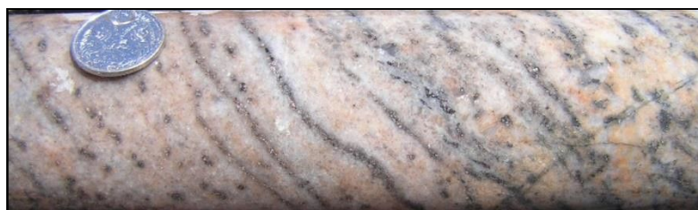
Figure 48: Gneissic pegmatite/leucogranite at 275.8m, DD16JUP004
