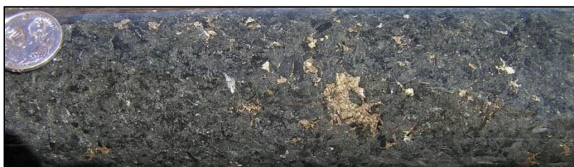
Figure 43: Massive gabbro containing interstitial pyrrhotite and pyrite at 194.8m, DD16JUP004
