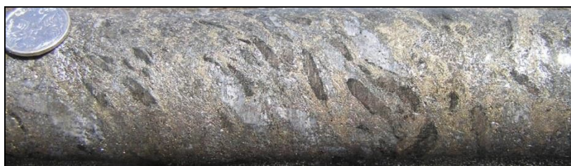
Figure 47: Pyrrhotite-matrix breccia with aligned clasts of graphitic schist and gneiss at 239.3m, DD16JUP004
