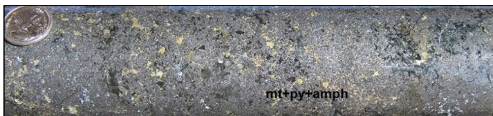
Figure 29: Massive magnetite +pyrite +amphibole IOCG alteration at 249.9m, DD16TUR016
