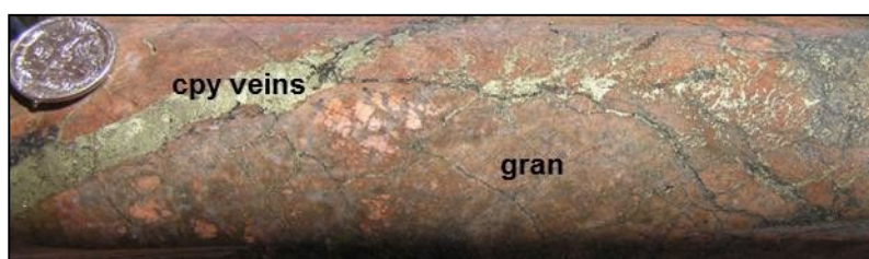
Figure 35: Chalcopryite-rich vein and wispy veinlets within leucogranite at 378.95m, DD16TUR016
