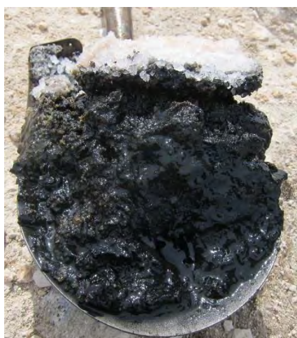
Plate 12-2: Hyposulfidic clay soil with monosulfidic material – Pond PA4d March 2014
