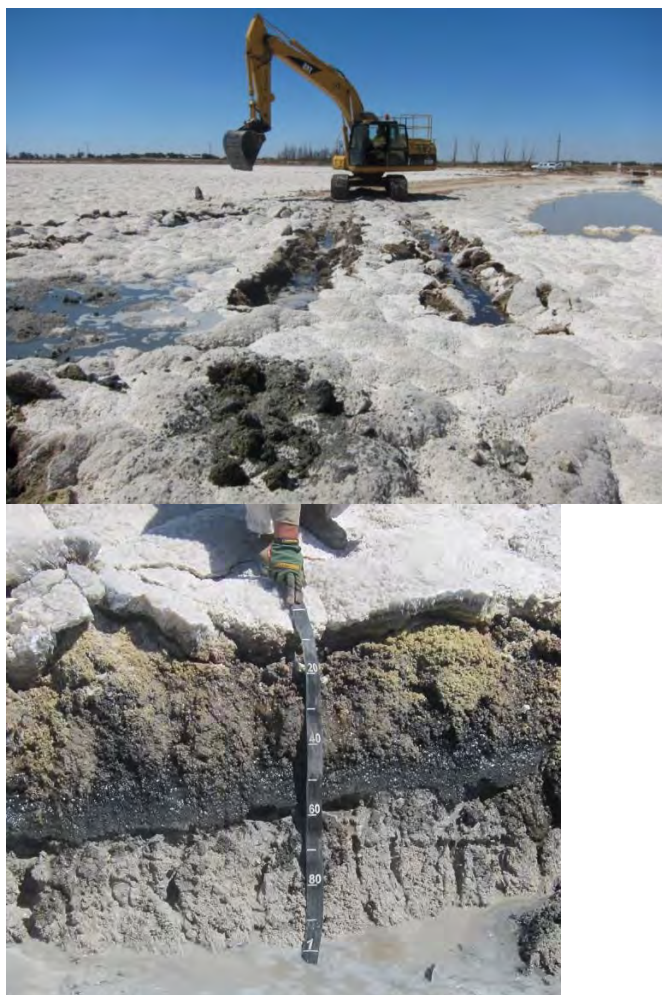
Plate 12-1: Gypsum crust – Pond PA7 Section 2 December 2013
