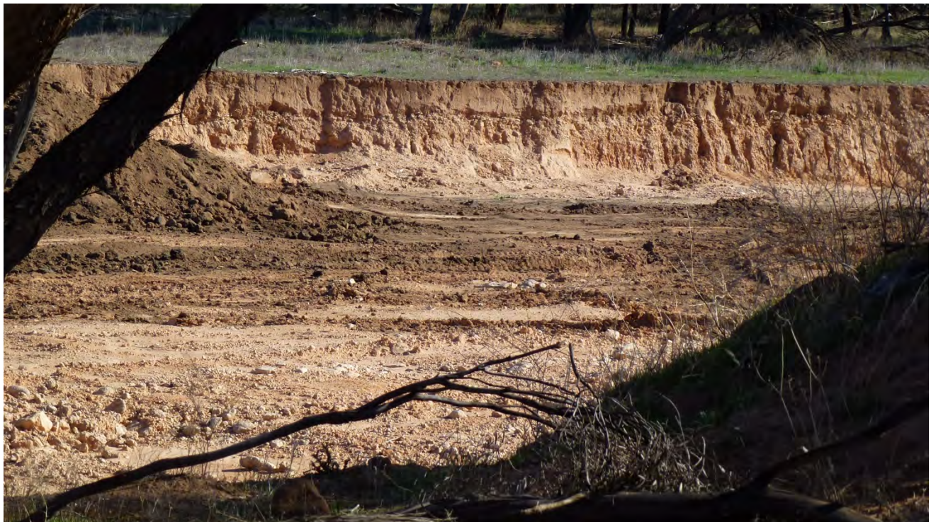
Photo 12: Detail of the subsoil near the location of the infiltration test Clean sand with little fine content, medium permeability.
