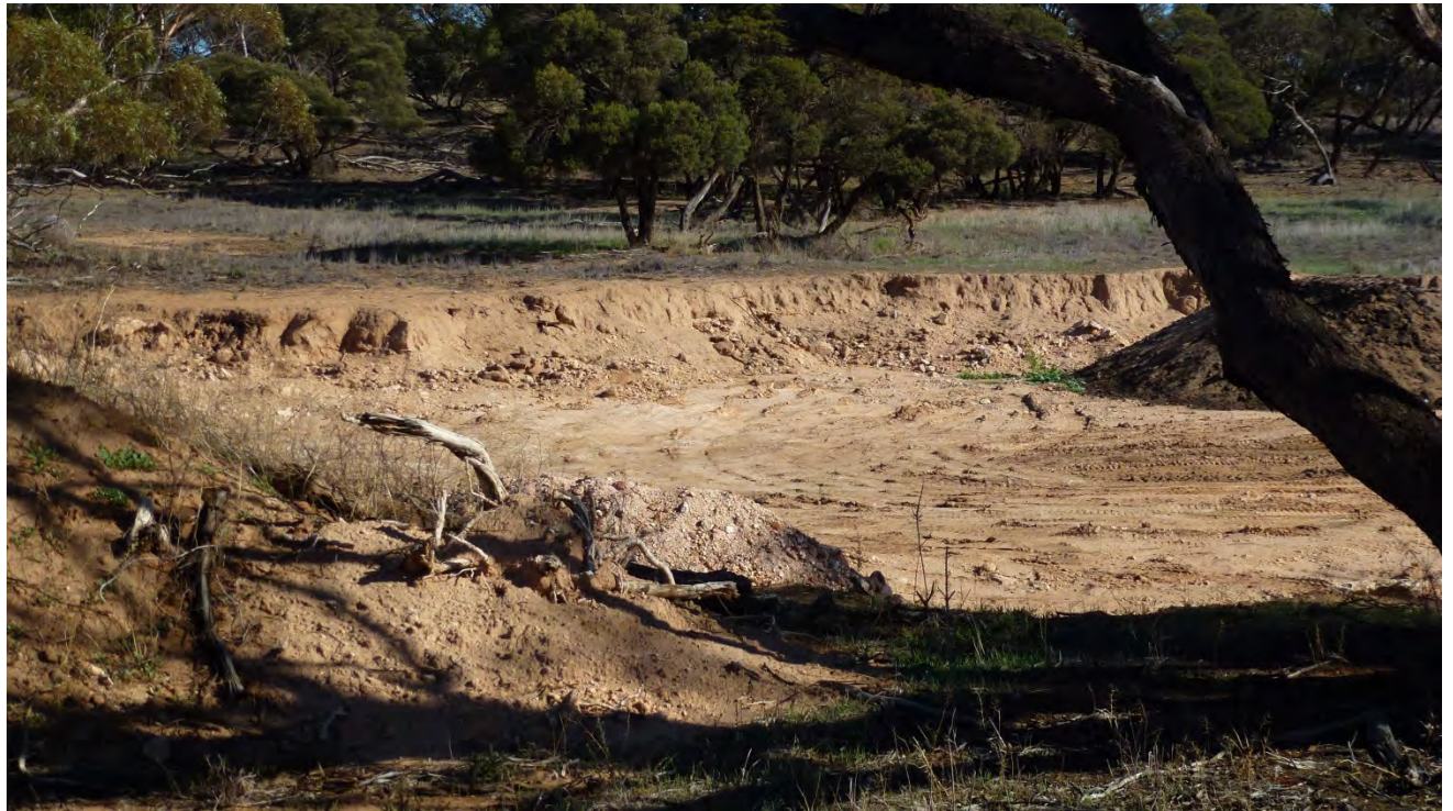
Photo 13: Detail of the subsoil near the location of the infiltration test Sandy loam with some non-plastic fines, low permeability
