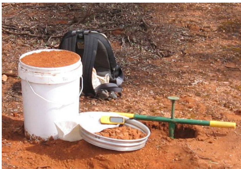
Figure 3: Sieving +6.4mm fragments from the regolith. Most of the oversize is calcrete or barren rock.
