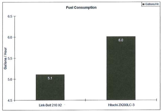
Fuel consumption was measured utilizing a calibrated fuel meter installed on each machine. Machines were operated in the highest work mode setting, running at the highest engine RPM, with 100% utilization.
