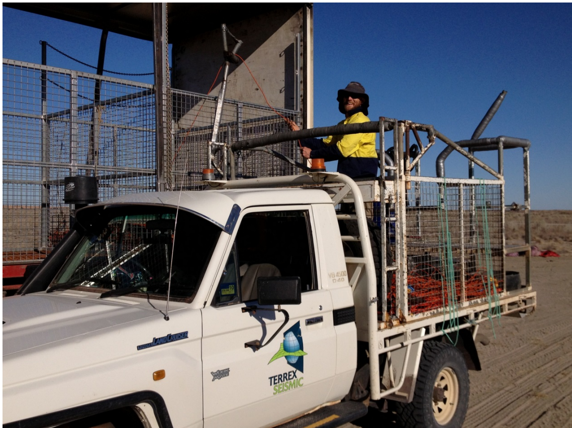
Photograph 2 - Cable truck pulling cable from the spread trailer
