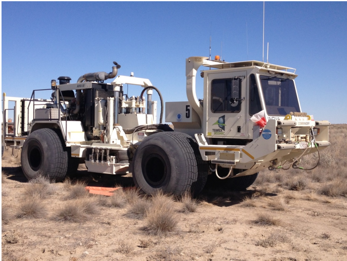
Photograph 1 - Vibrator ready for refuelling in the field with orange spill mat under the machine
