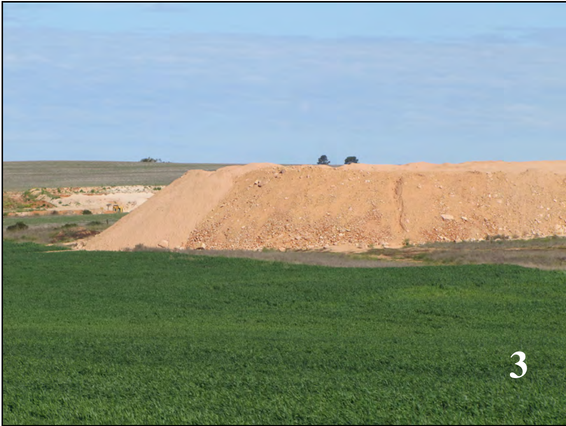
VIEW OF OVERBURDEN DUMP (20,000m 3 ) IN PROGRESS TO BE USED IN BACKFILLING FOR REHABILITATION
