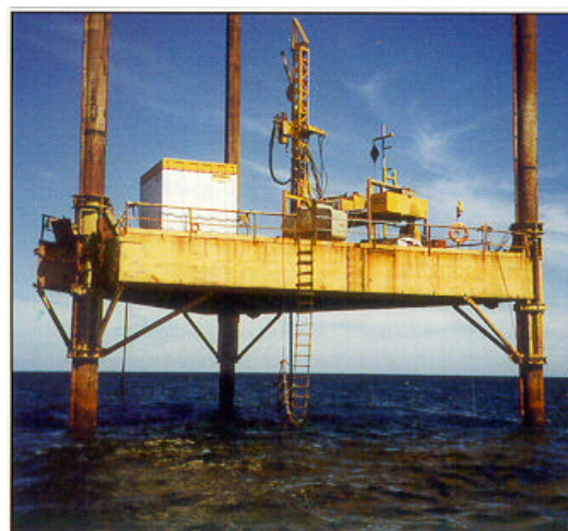
Jack-up platform on location in Spencer Gulf. (Photo 44504)
