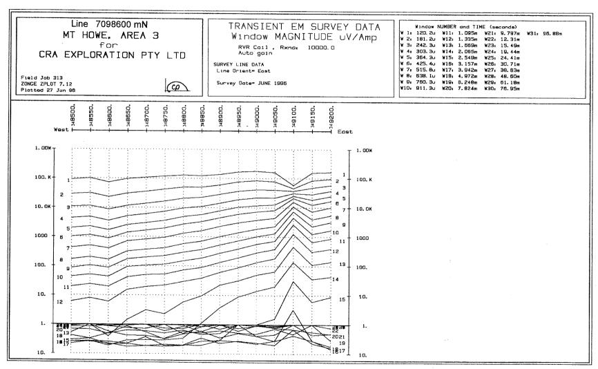
\* Twin Turn 200m x 200m Transmitter Loop \* 50m Stations
