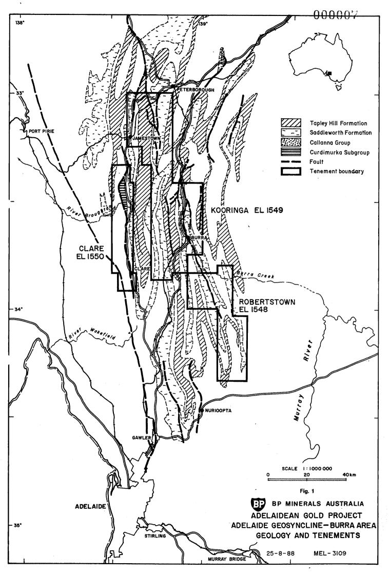
The simplified lithostratigraphy of the tenement, taken from Mirams (1964) and Thomson (1969), is summarised in Table 1. The primary target units are those containing calcareous or dolomitic members; secondary targets are carbonaceous or pyritic units. Massive sandstone units, greywackes, turbidites, siltstones or tillites have not been targeted for sampling.
