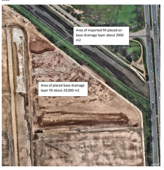
The next figures show that the fill as placed in the 200 m2 area reached an elevation of about 9 m AHD above the top of the base drainage layer at about 3 m AHD. The level information from Nearmaps is very approximate. The impression from the photo of the fill mound (see further below) is that the top of the mound is more like 4 m above placed base filter / drainage layer – not 6 m.
