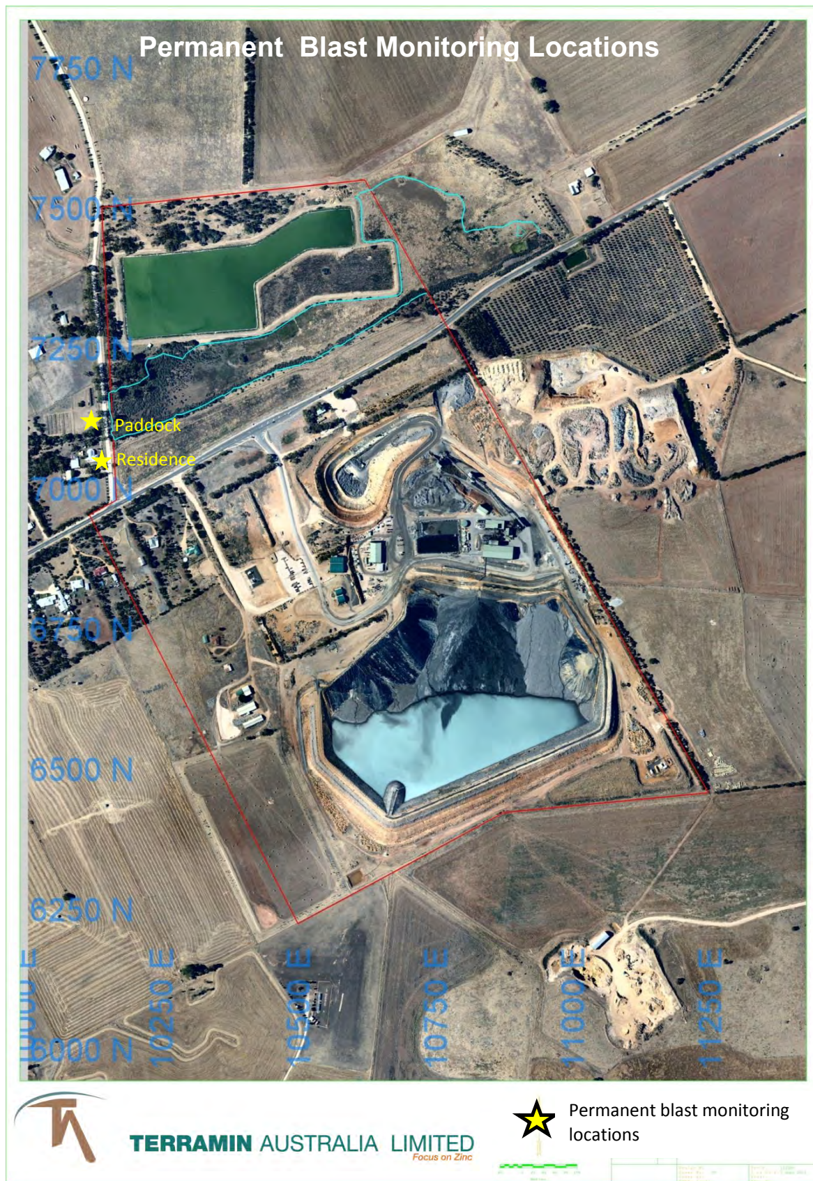
Figure 43: Fixed Blast Monitoring Locations
