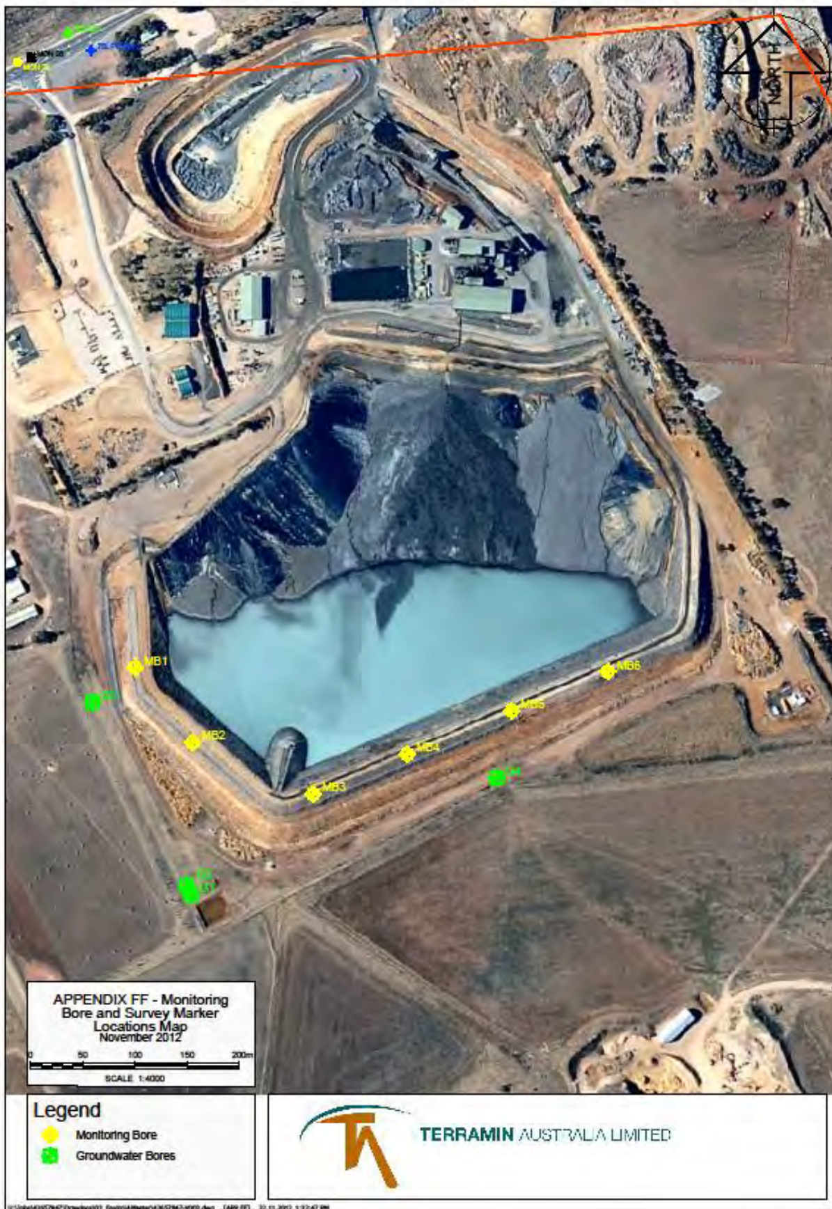
Figure 42: TSF Embankment Bores Monitoring Locations
