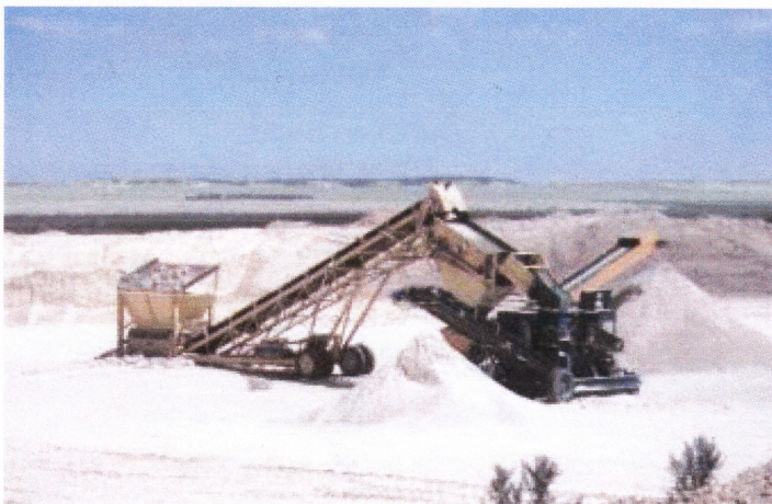
Gypsum screening plant at the Everard deposit. (Photo 47716)
