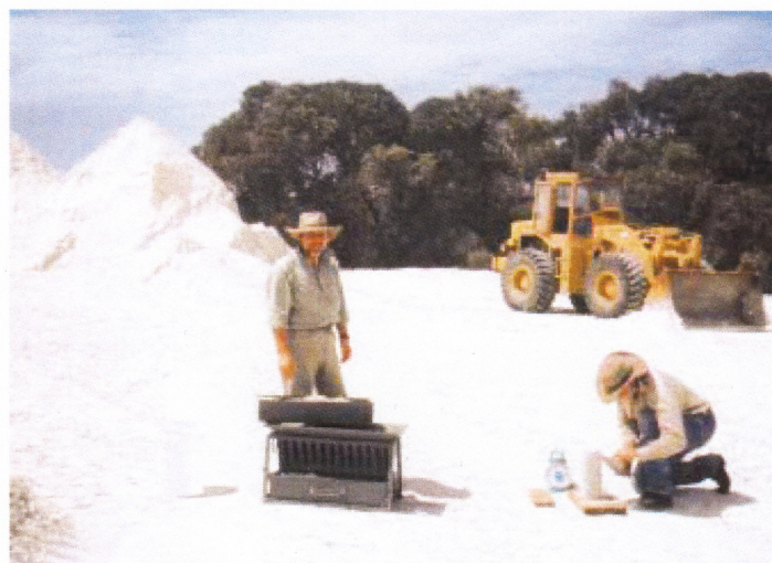
Splitting and weighing gypsum samples at Elephant Lake. (Photo 47712)
