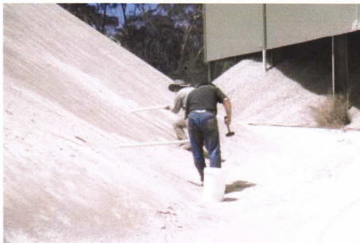
Sampling stockpiles of gypsum from the Blanchetown deposit. (Photo 47714)
