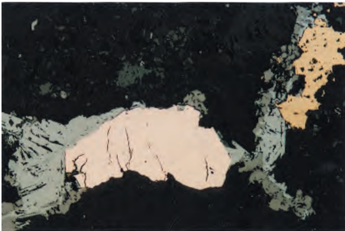
Fig 25 QBE#1, 403.4m 0.09 mm PS (x100) Ore mineral veins also in this sample, with typical composites of pyrite, chalcopyrite associated hydrothermal hematite (pale grey) and magnetite minor grey-brown granular.
