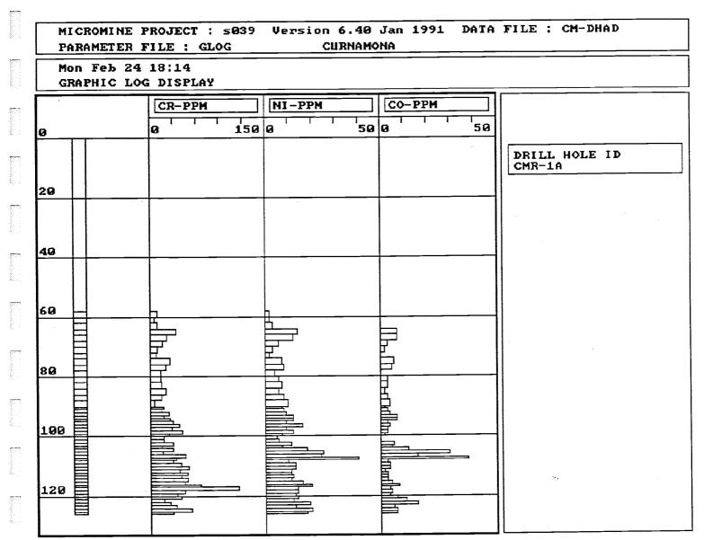
DATA FILE : CM-DHAD Version 6.40 Jan 1991 MICROMINE PROJECT : s039 **CURNAMONA** PARAMETER FILE : GLOG Mon Feb 24 18:17 GRAPHIC LOG DISPLAY P-PPM MO-PPM FE-% 1000 20 0 100 ø DRILL HOLE ID CMR-1A 20 40 60 80 100 120
