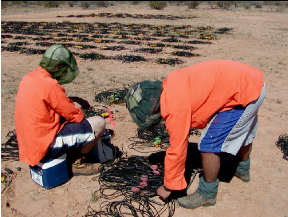
Picture # 4- 2: testing geophones prior to the start of the Albus Seismic Survey
