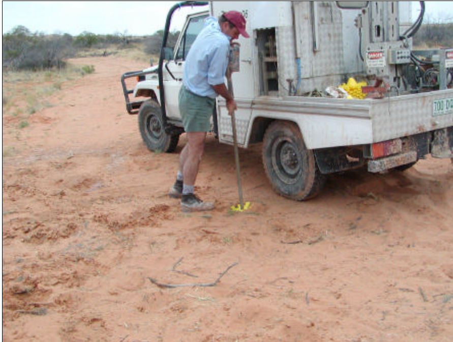
Picture # 5- 3: Expertest Observer Don Blick pushing a hole-hat into a restored uphole.
