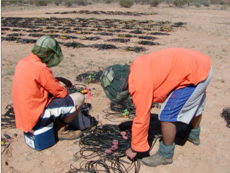
Picture # 1: testing geophones before start-up.
