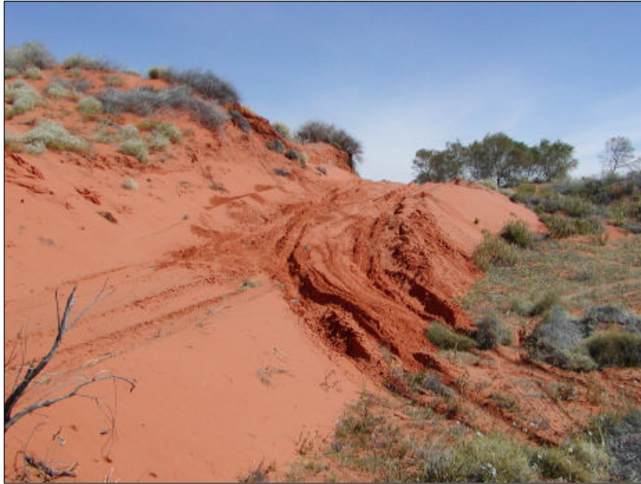
Picture #6- 6: dangerously soft side cut on line BC03-07; the recording truck slid off the side of this cut while reversing out of soft sand.
