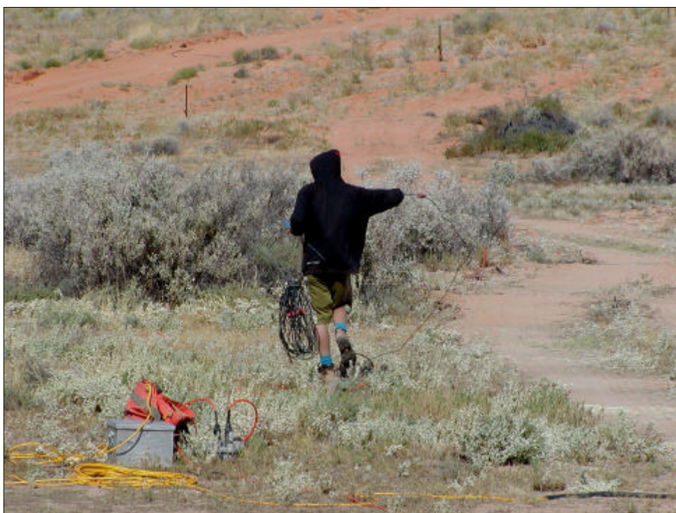
Picture # 4- 5: picking up geophone on Line BC03-22 near the fence line
