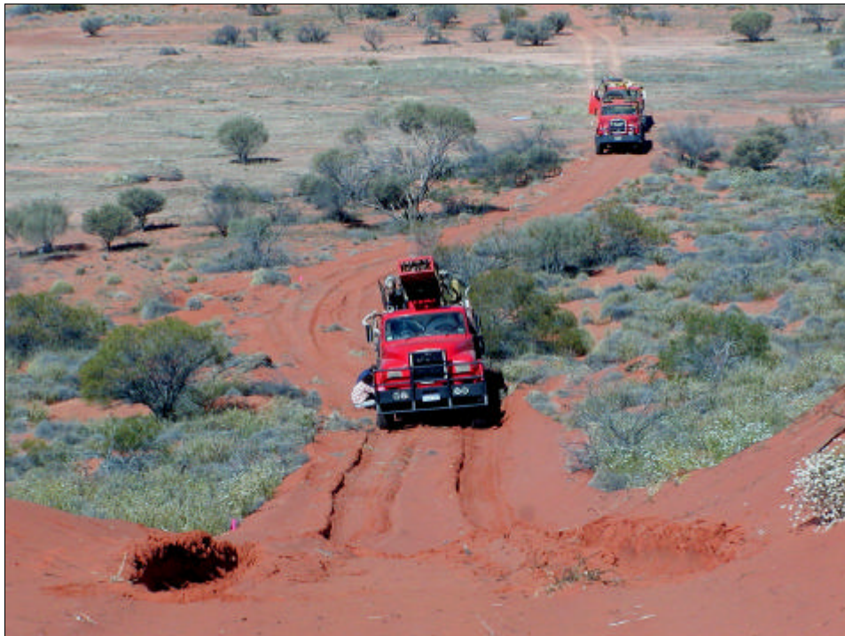
Picture # 5: reducing rig tyre pressures in order to get over a steep soft dune on line BC03-09
