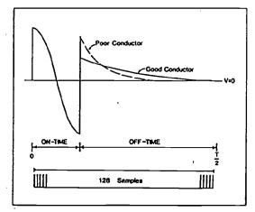
Figure 2B Sampling and Wave Form
