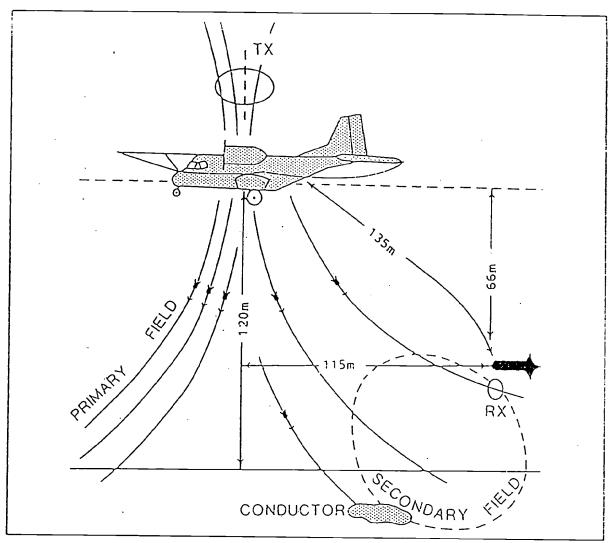
Figure 2A System Geometry
