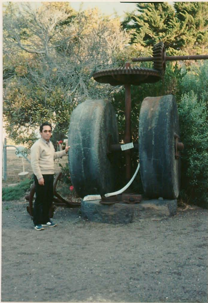
PLATE 1. Basalt pan mill used to crush pegmatite mined between 1905 to 1910. Penneshaw May, 1987. Slide No. 36104
