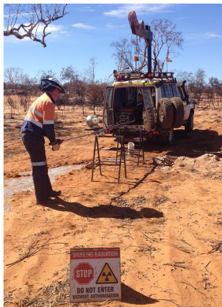
Figure 3. Example of logging truck exclusion zone during radioactive source handling.
