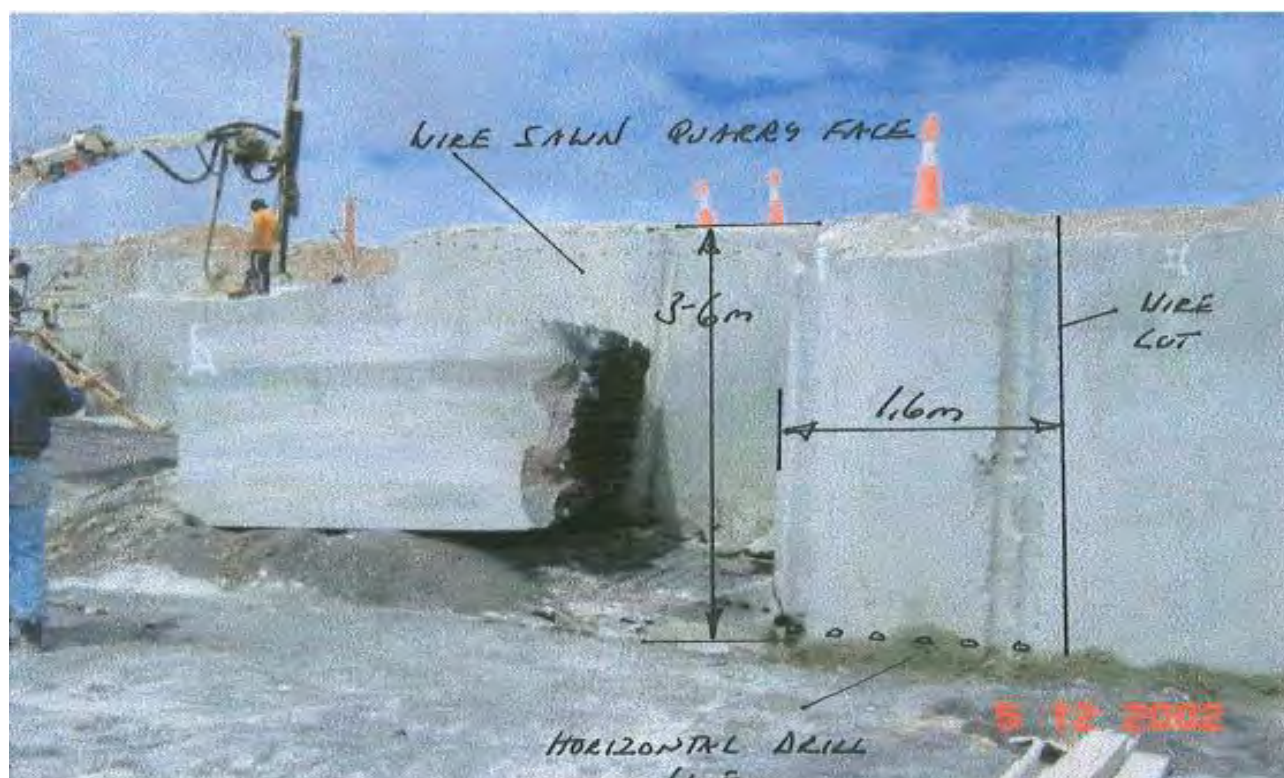
Plate 8 – Annotated image of dimension stone mining method from ADP 2000/073
