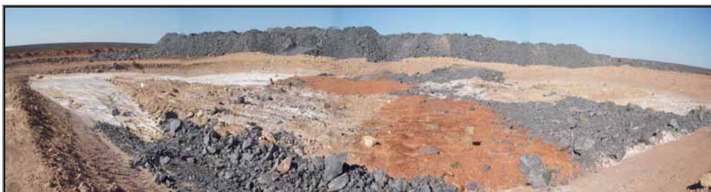
Plate 3 - Looking west on to Challenger's tailings capping trial which shows limited vegetation establishment (Feb, 2007)
