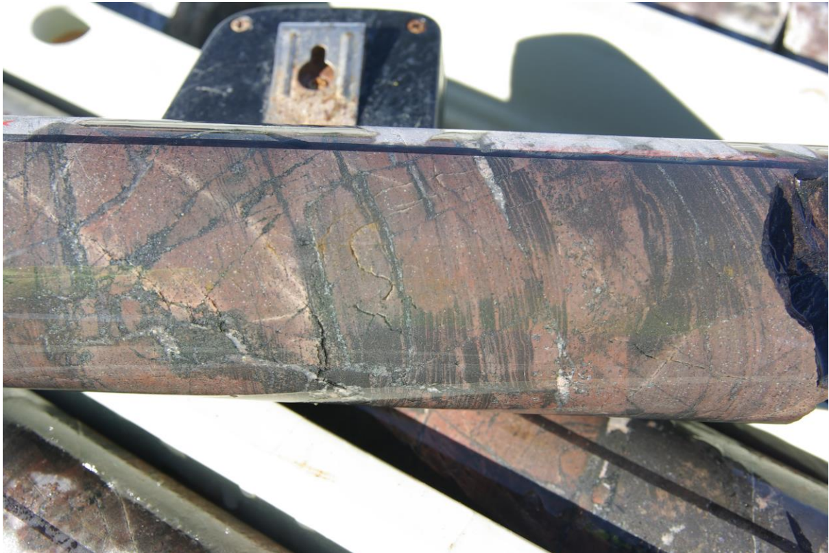
Intense fine magnetite replacement fronts emanating from around fine magnetite (+carbonate-pyrite) veins. 198.7m.
