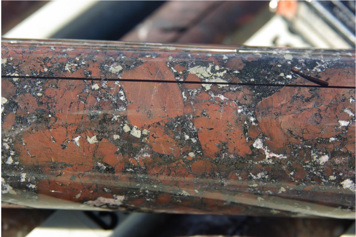
Plate 1: Extensive brecciation, wall rock alteration, magnetite veining and patchy pyrite
