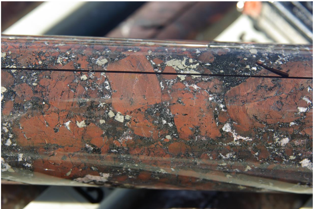
Breccia of "red rock" -magnetite altered albitite with magnetite+-(biotite/amphibole-carbonate-pyrite infill. 306.4m.
