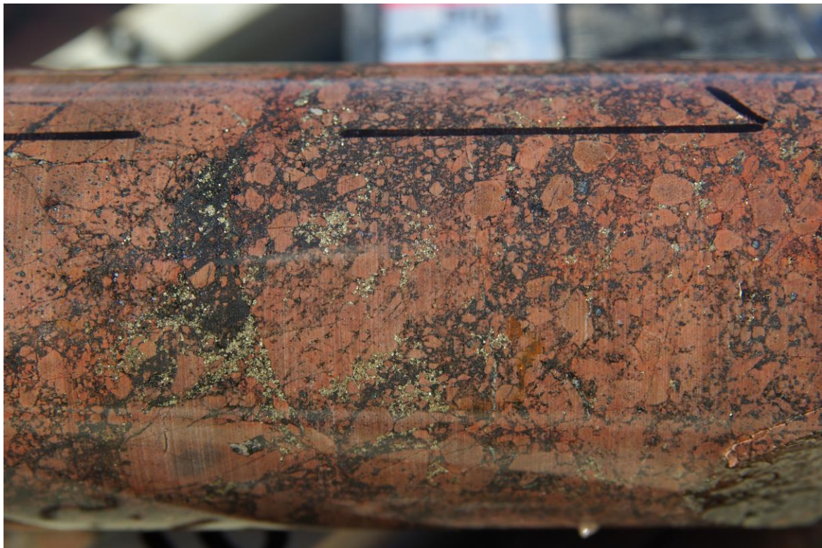
Plate 2: Magnetite veining infill of fracture system in altered metasediments
