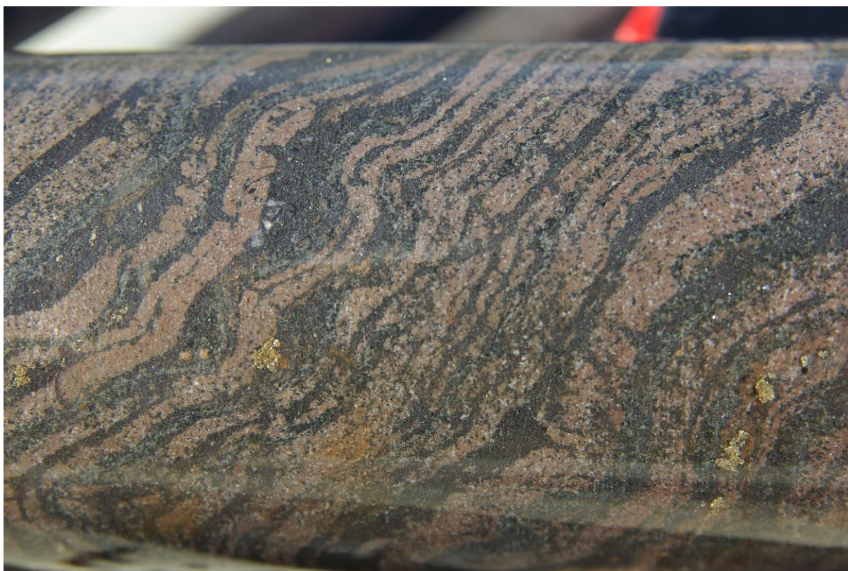
Magnetite (+-pyrite) replacement and infill of suspected carbonate beds. 114.1m.
