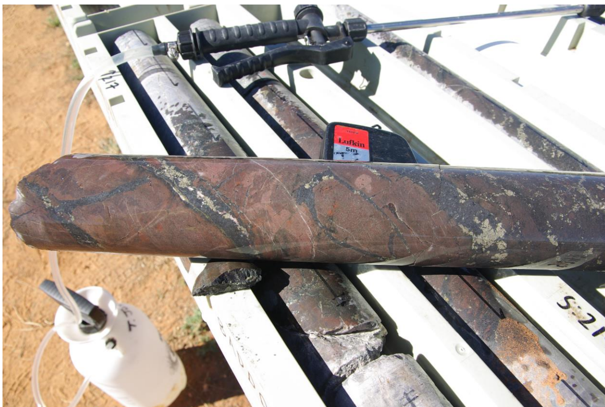
Network of thick magnetite-pyrite veins and associated fine disseminated replacement in and orthogonal to bedding. 215.6m
