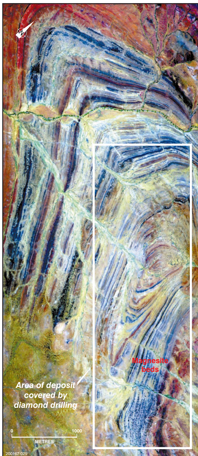
Fig. 2 HyMap image of the Witchelina magnesite deposit delineating magnesite lithology (blue colour) and structure.
