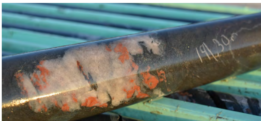
Figure 4-2: Large irregular leucosome with hematite dusting of alkali feldspar in magnetite rich BIF with disseminated euhedral specular hematite porphyroblasts (CY15-002, 191.30m).
