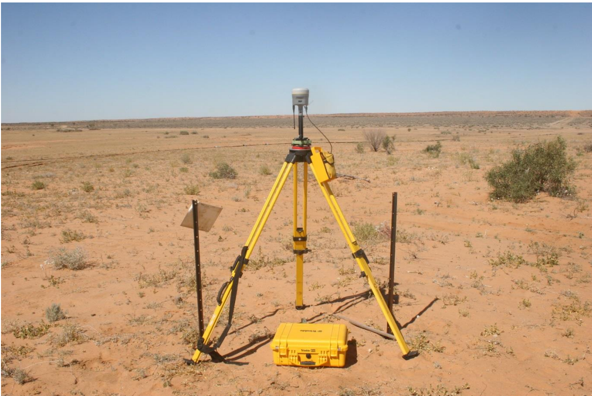
Photograph 1 Trimble R10 on CON6 control station (Fyfe benchmark)
