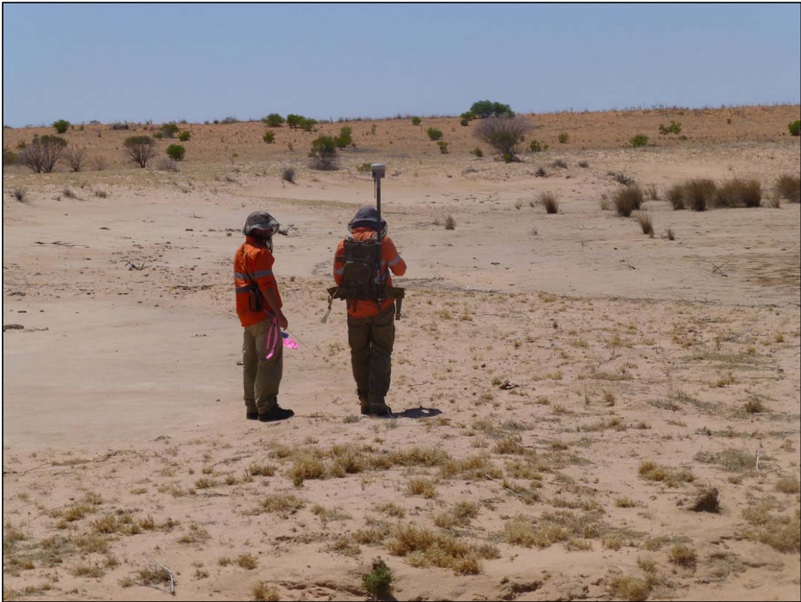
Survey staff using the Trimble R10 GPS back pack to survey the hand carry sections on receiver lines
