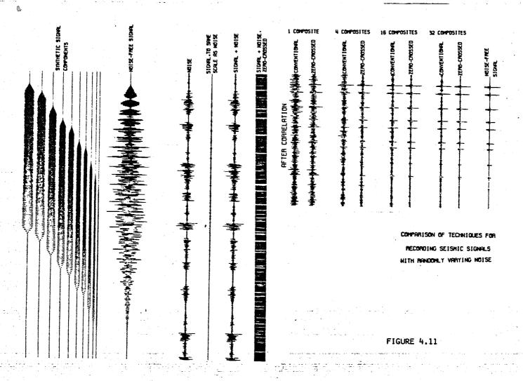
the one bit recordings have a superior signal-to-noise ratio. The difference is maintained through all comparisons up to 32 composites and clearly, the relative amplitudes have been preserved reasonably well.
