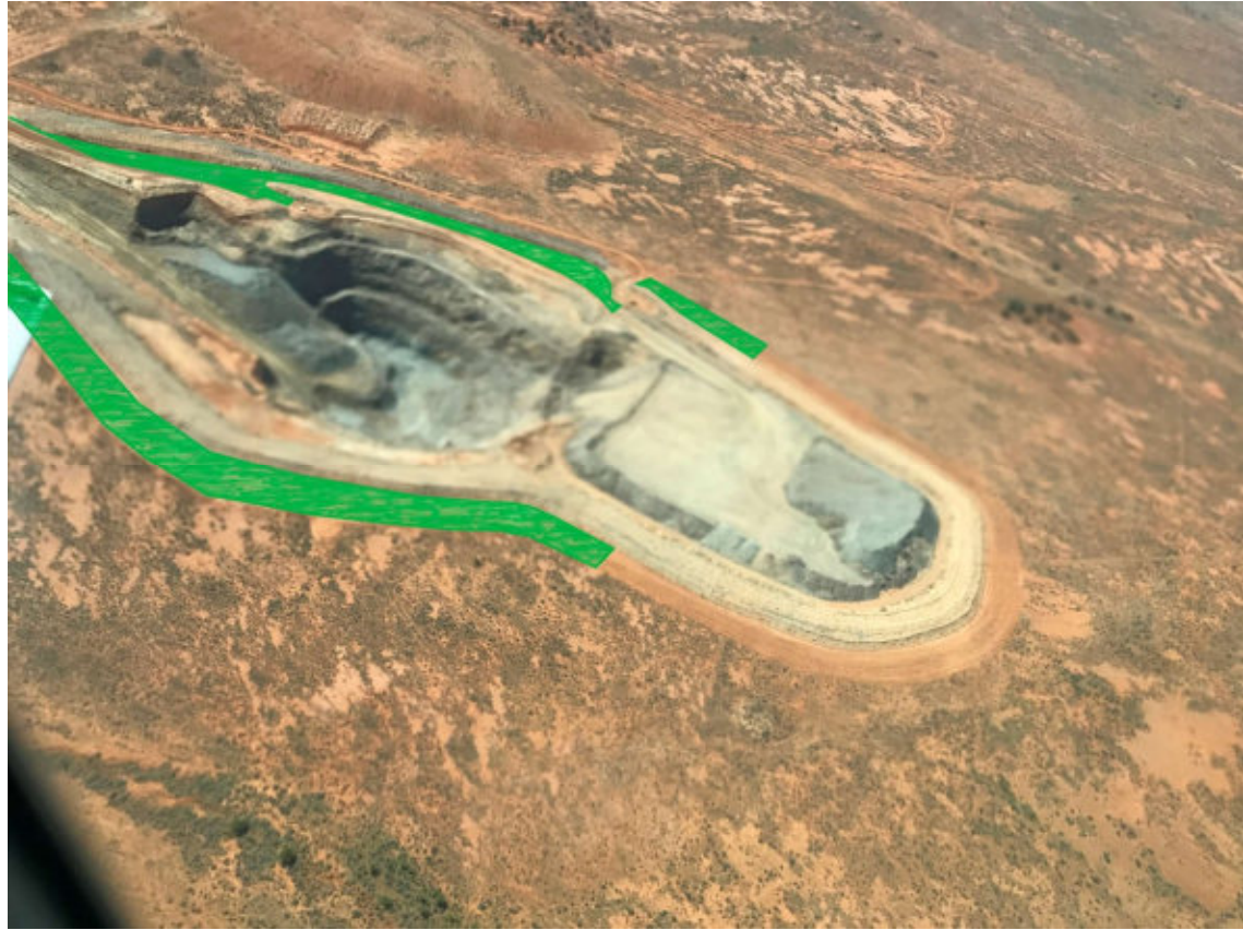
Figure 15: Vertigo roads and pit apron ripped and seeded (green)
