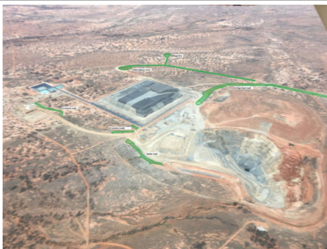
Figure 13: Haul Roads and laydown areas rehabilitated (ripped and seeded in green)
