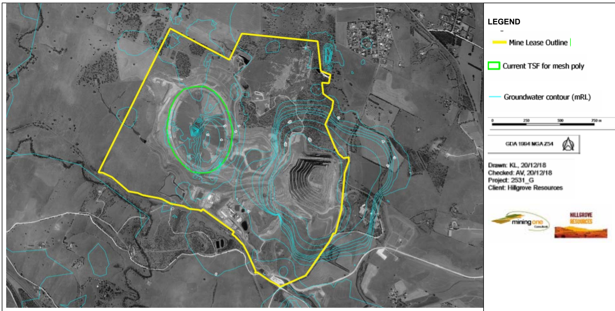
Figure 5-2 – Difference in groundwater head in 2023 between no underground and underground + TSF level 1266m RL (Stage 8)
