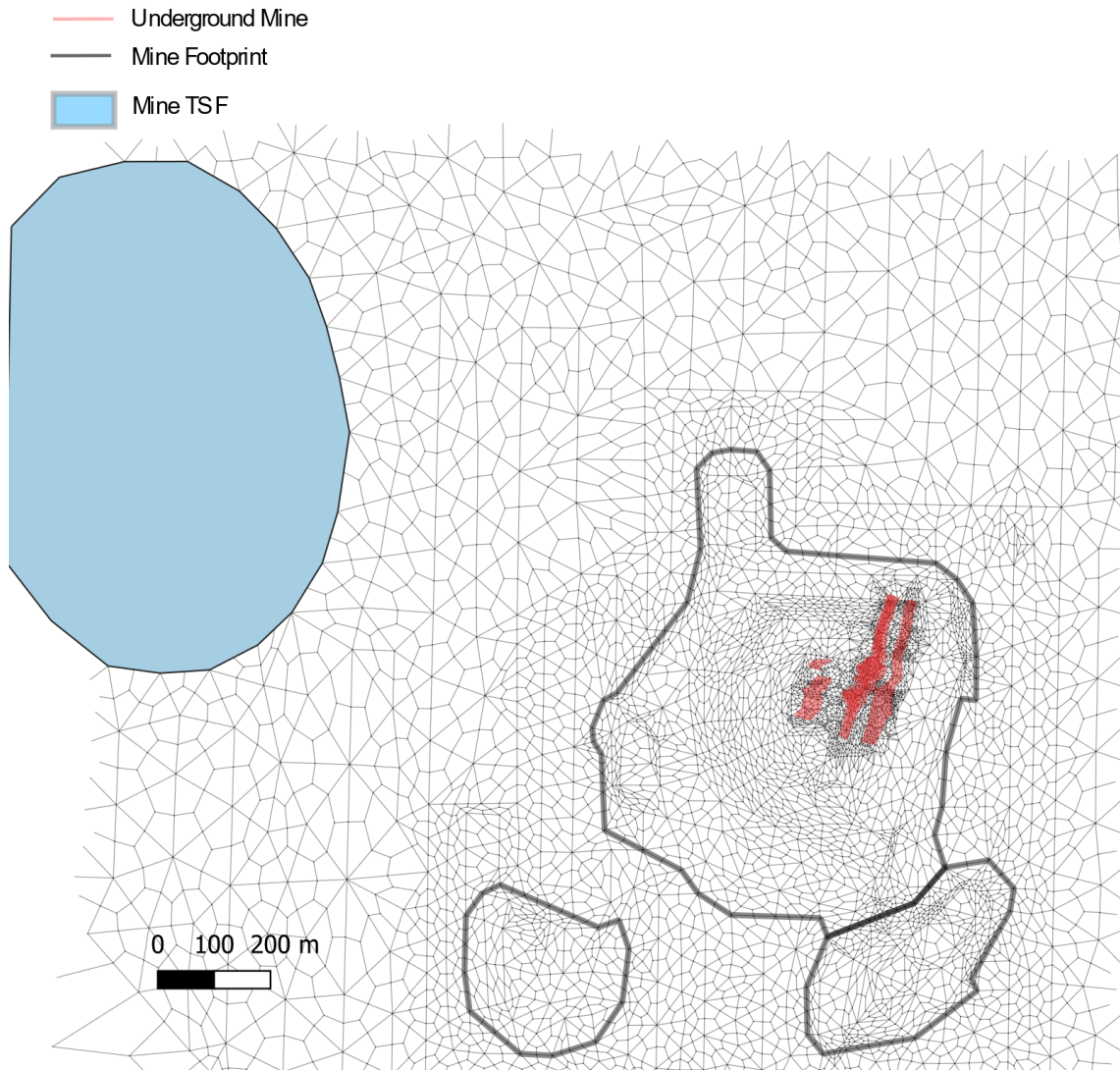
Figure 3-3: Refined Mesh with Location of Underground Mine Extensions (from Left to Right OB2, OB3U, OB3L, OB9 & OB10), Open Pit Mine Footprint and TSF
