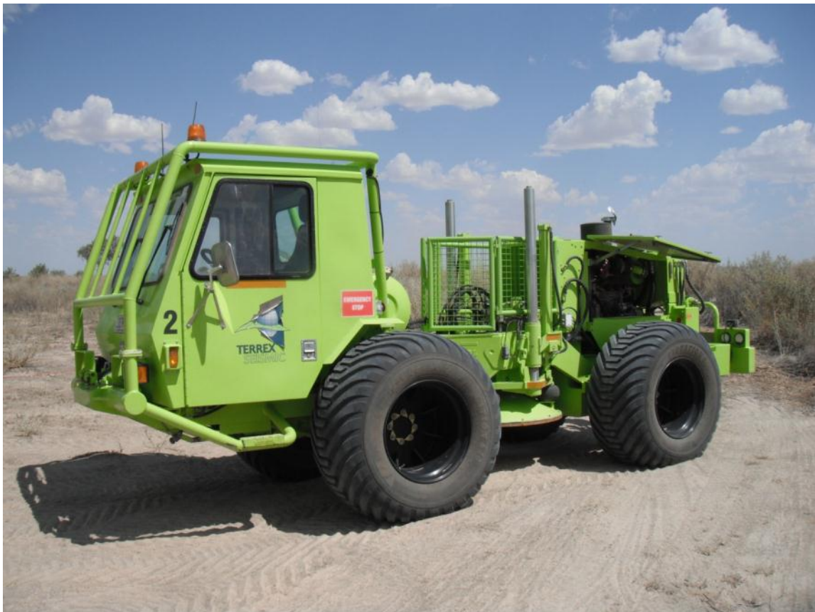
Photograph 2 – Envirovibes were used during sweep tests
