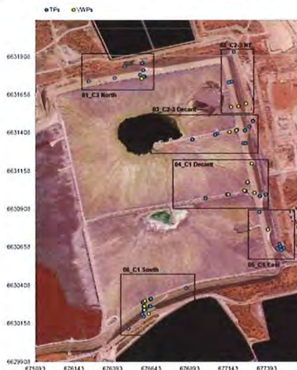
Figure 66: TSF 1-3 piezometer locations
