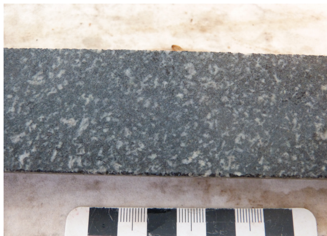
2(b) Weakly foliated hornblende-quartz-plagioclase-biotite gabbro, 188.5–189.6 m, drillhole DD89EN 46 (drillhole number 141782). (Photo 417828)
