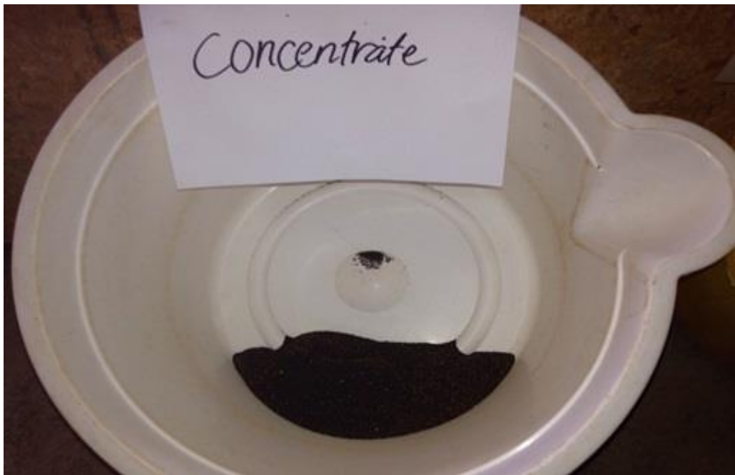
Photo 2 - Concentrate produced by Magnetic Separator
