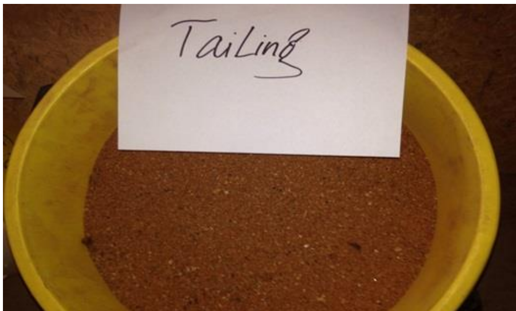
Photo 3 - Tailings produced by magnetic separator
