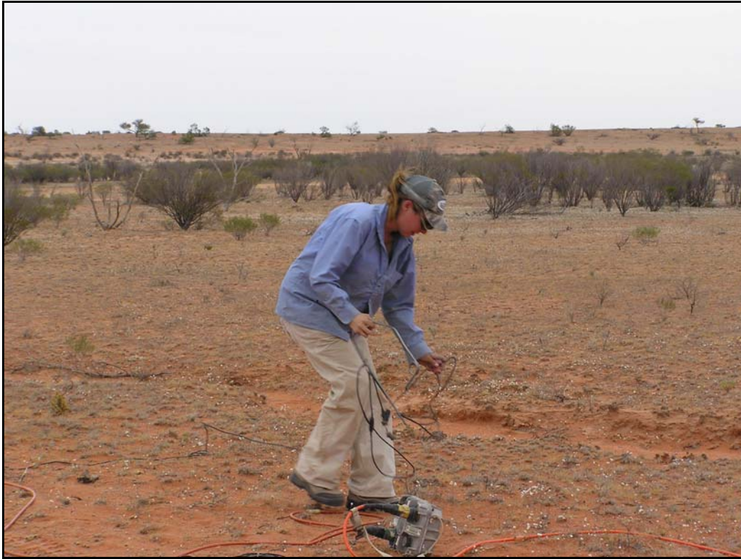
Picture 8- 1: juggy Sarah Anderson stomping geophones on line BC05-50 in PEL 95 a few days before she suffered burns to the left ankle that ultimately led to a career change to a cable and geophone repair person.
