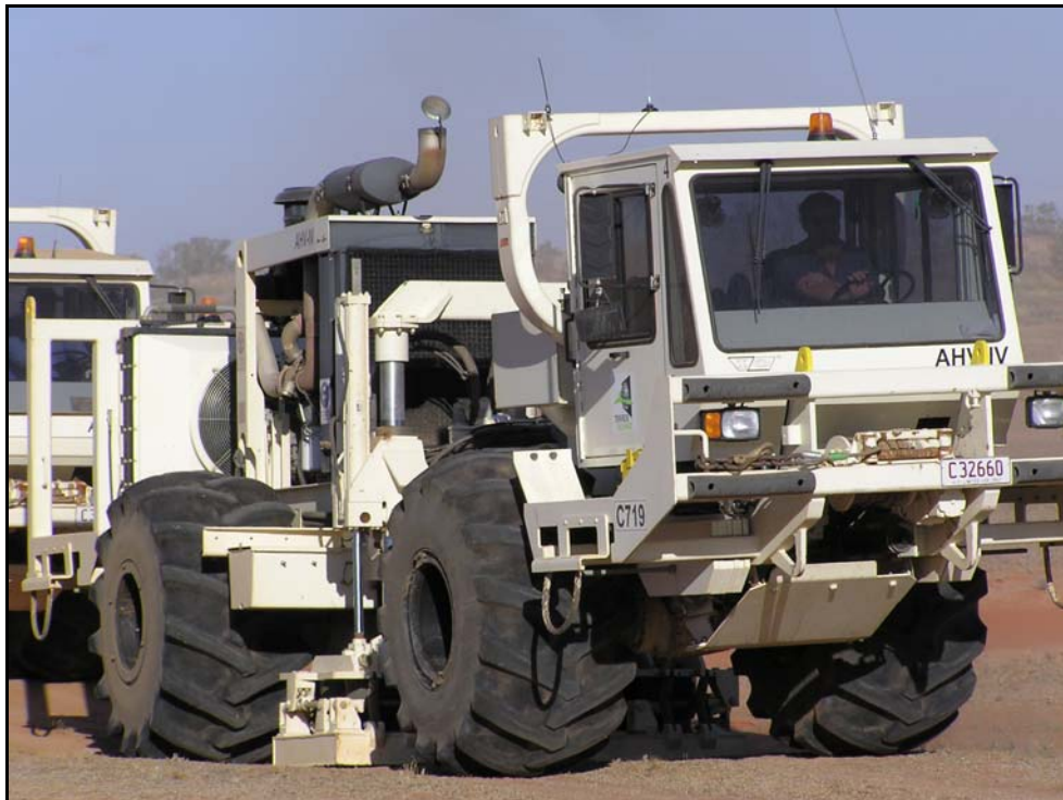
Picture # 5- 5: the I/O AHV IV vibrator with the heavy lug tyres.
