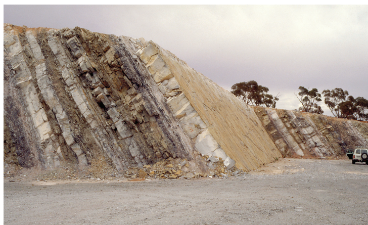
Figure 7 Myrtle Springs quarry in interbedded dolomite (grey-pale brown) and magnesite (white); magnesite bed 5 cleaned and ready for precision blasting and extraction in 1998. (Photo 046337)
