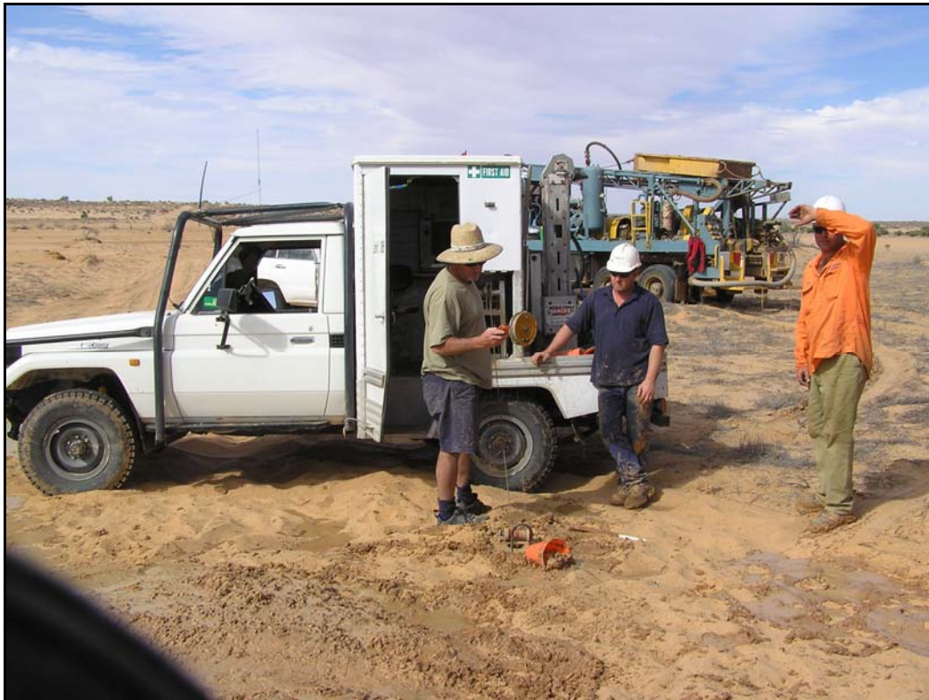
Picture # 6- 3: Expertest logger Mark Smale (left) loading the tool in the hole and watched by the drillers to see that there are no problems
