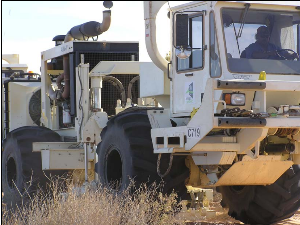
Picture # 9- 1: the I/O AHV IV vibrator; large lugs on the tyres are inappropriate for sand
