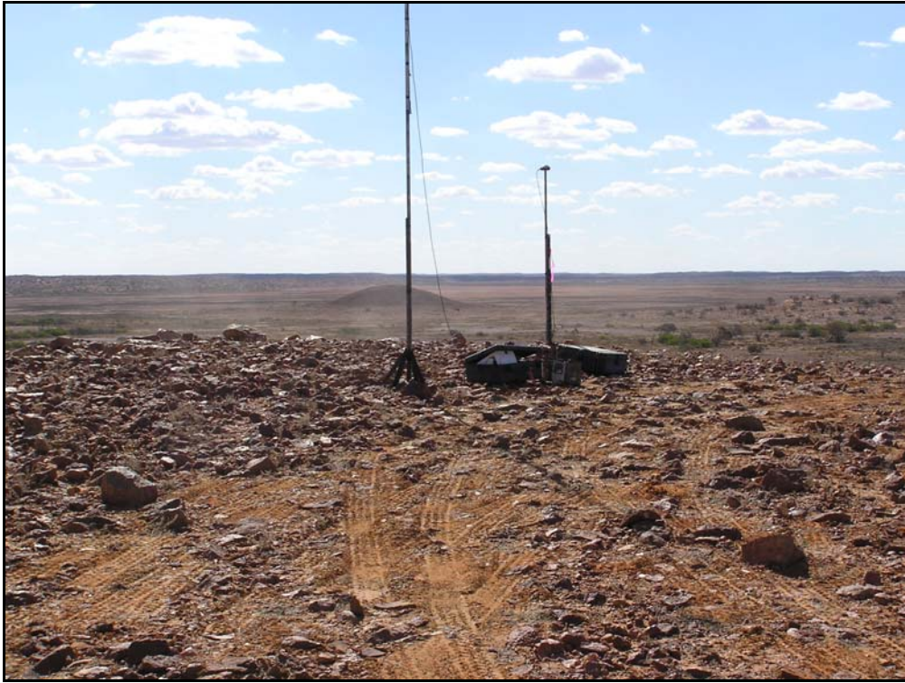
Picture # 7- 9: DSS base station on a gibber jumpup in the Boomer area
