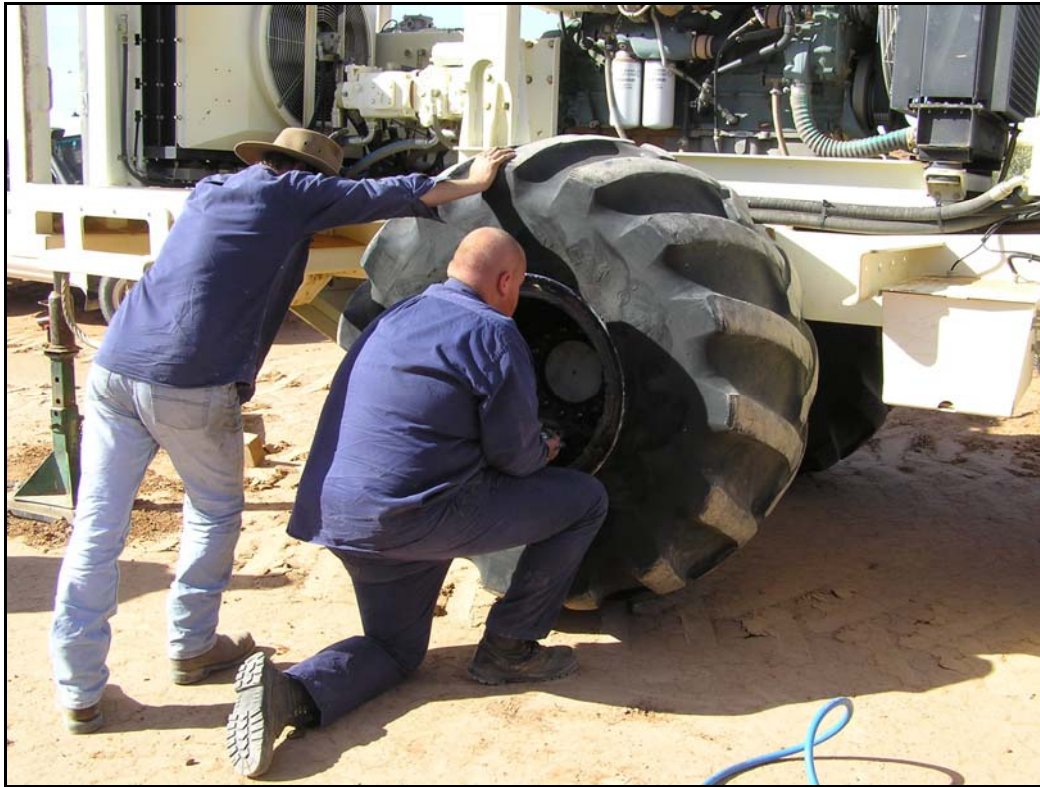
Picture # 5- 7: vibe tech Shane Goosens (kneeling) and Richard Carmody change a vibe tyre. Note the large lugs, inappropriate for sand.
