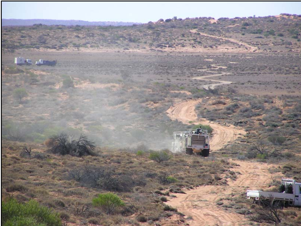
Picture # 5- 1: vibes on line BC05-16 with recording truck and vibe service truck to left
