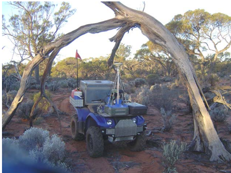
Photo 1: Quadbike used for gravity surveying
