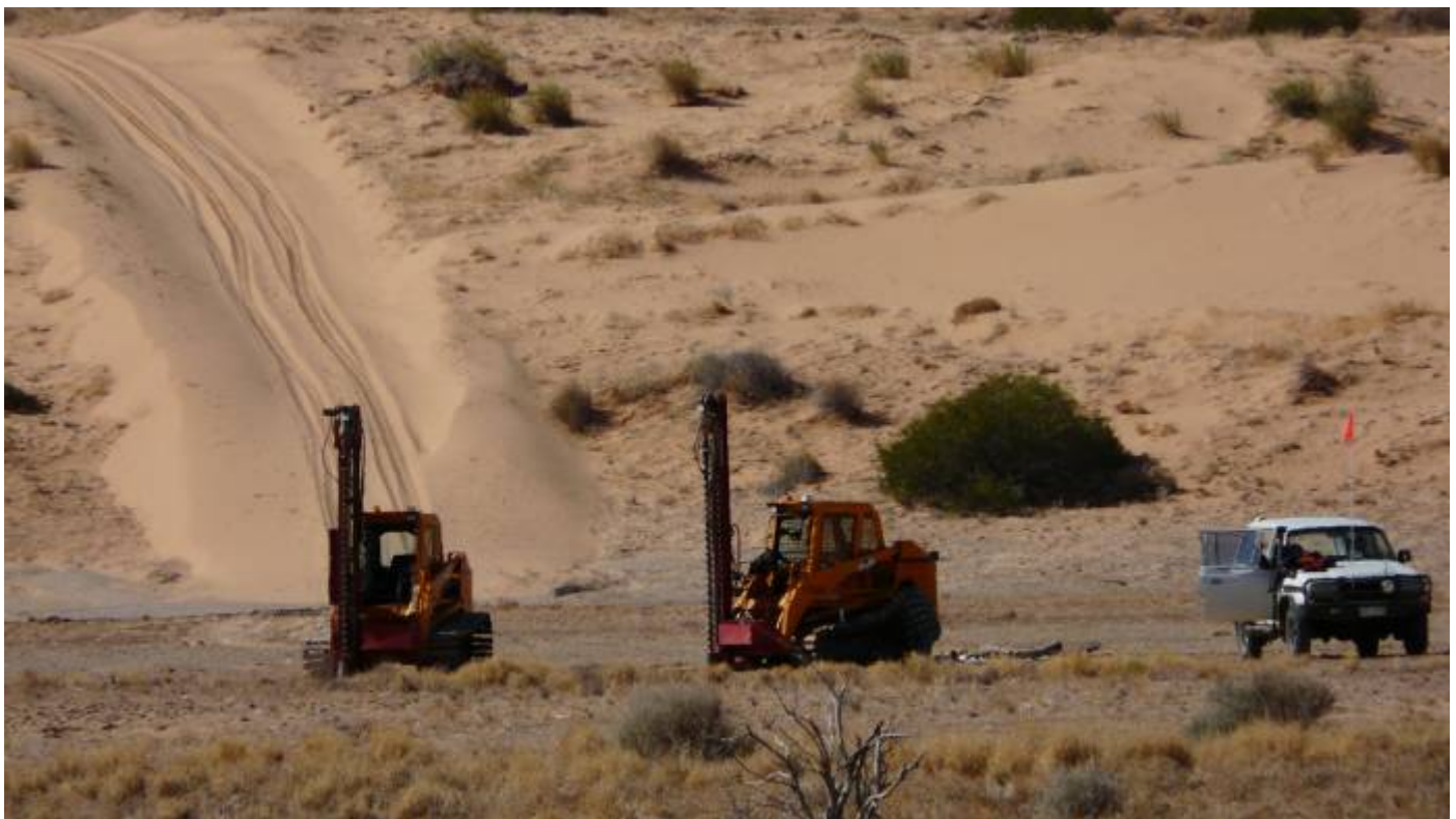
Bobcat mounted drill rigs used for drilling explosive shot holes
