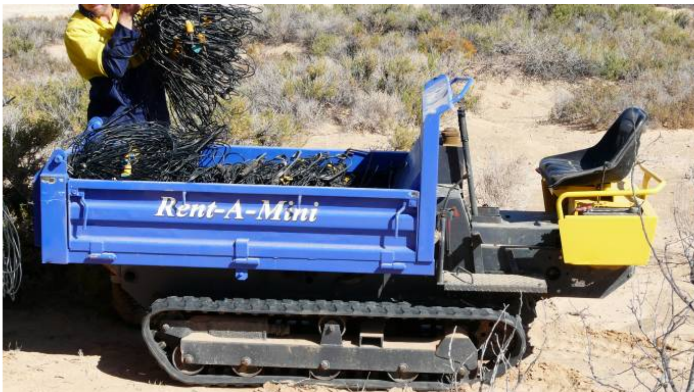
Yanmar tracked vehicles used by line crew to traverse salt lakes with spread
