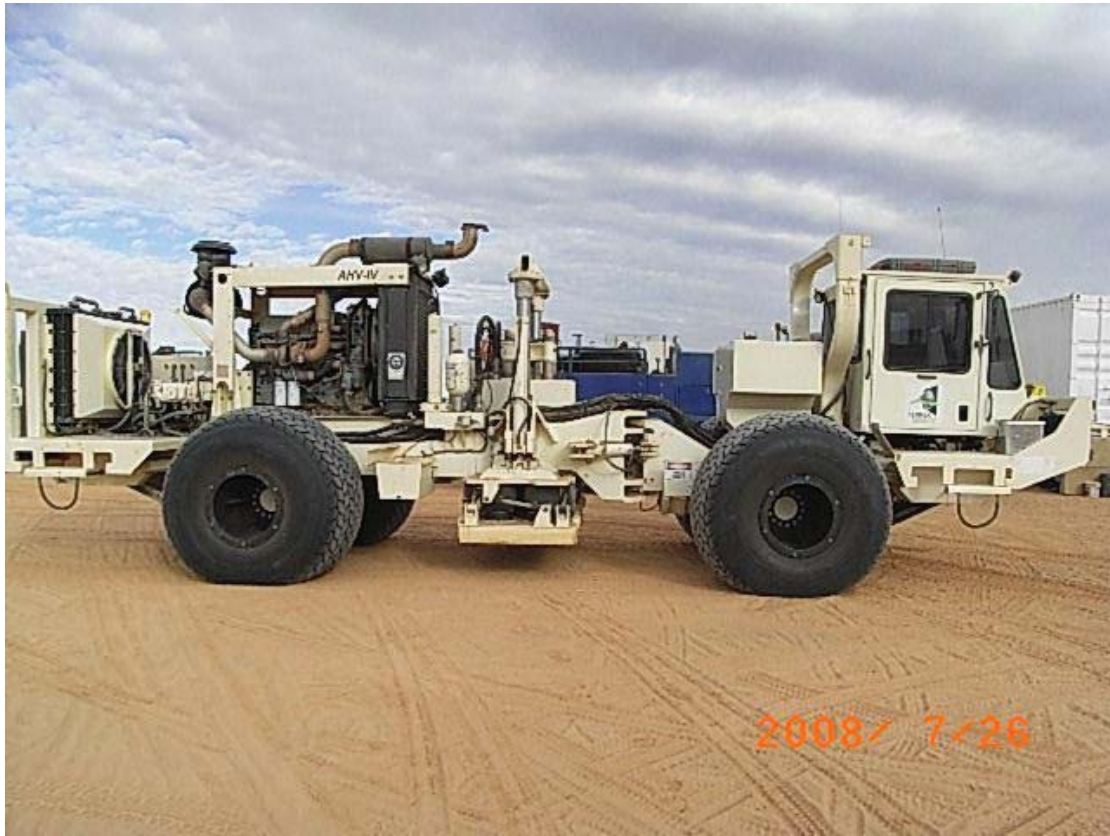
Picture # 5-3: I/O AHV IV Vibrator fitted with sand tyres.
