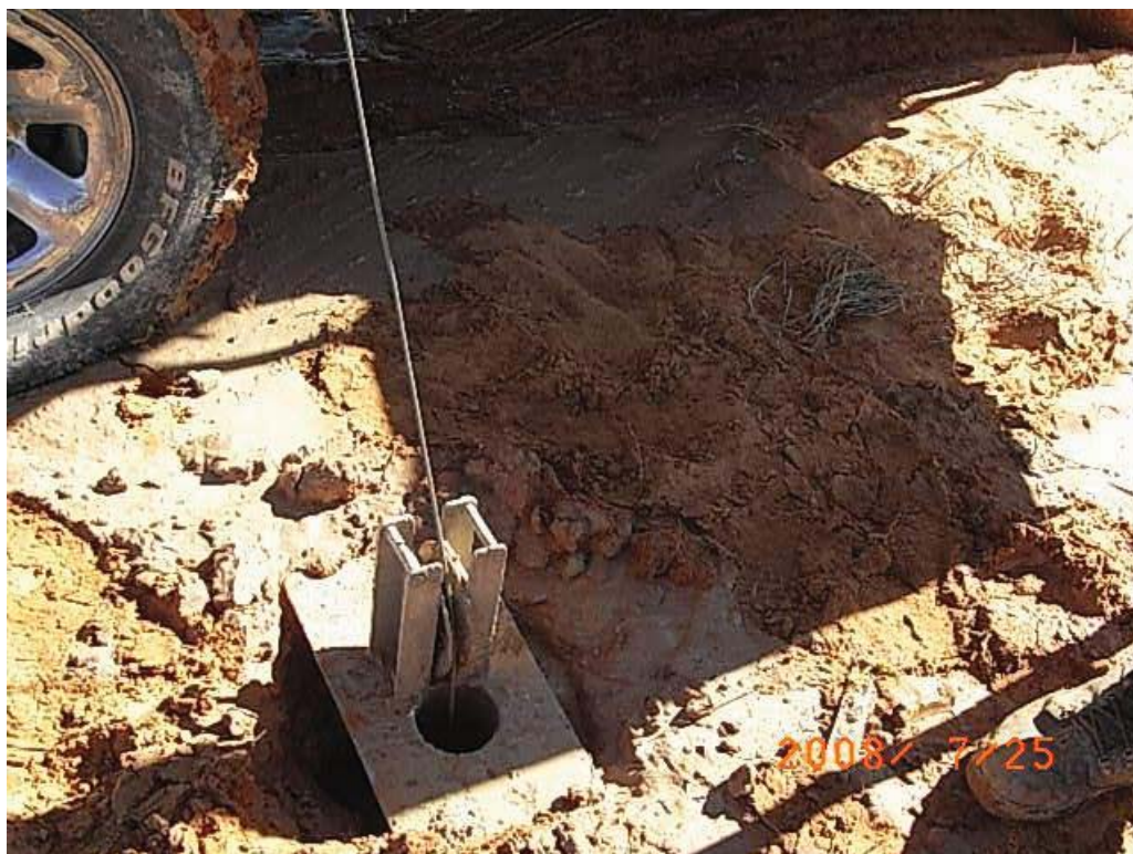
Picture # 6-4: Connecting cable to down-hole geophone.
