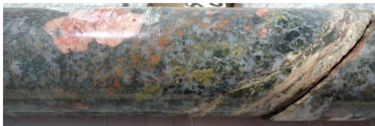
Figure 12: Epidote and chlorite alteration associated with calcite vein (745.4 m)
