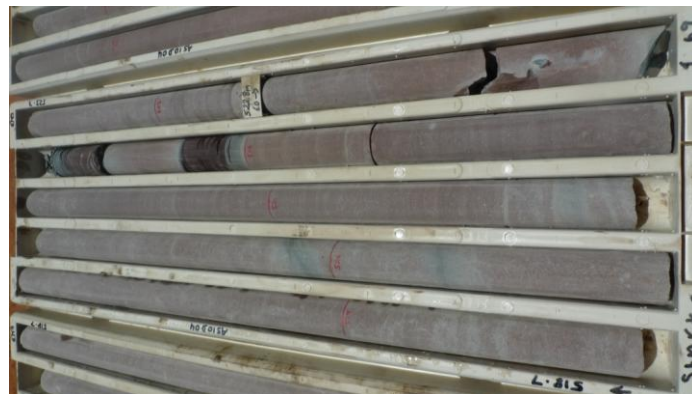
Figure 7: Tregolana Shale /Whyalla Sandstone? (518.7–523.3 m)
