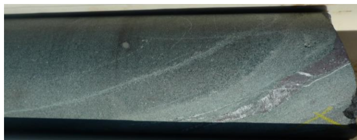
Figure 11: Minor haematite and calcite vein within dolerite dyke (712.4 m)
