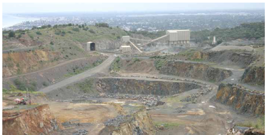
Figure 3 Linwood Quarry showing the view north to crushing plant and Adelaide city area. The quarry is located ~15 km SW of Adelaide CBD and produces limestone for aggregates, road base and rail ballast. (Photo 408319)
