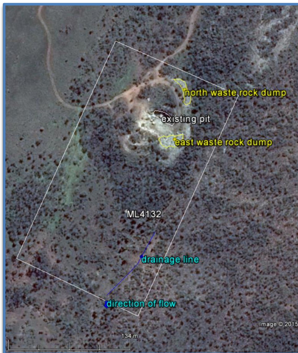
Figure 9: Mine Plan showing ML4132 boundary, existing pit, waste dumps to be mined and natural drainage
