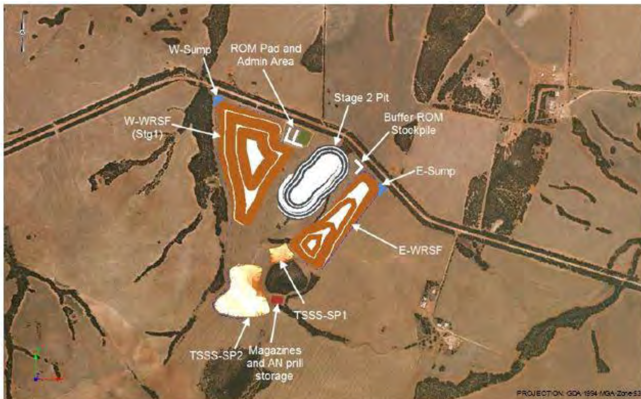
Figure 3-18: Pit and mining infrastructure - Stage 2 (AMC 2015)
