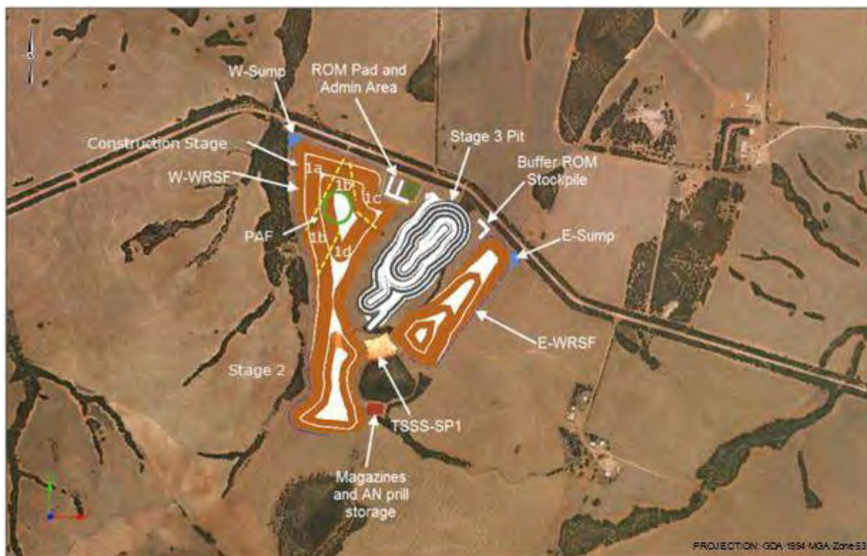
Figure 3-24: PAF cell with 250,000 tonne capacity within the western WRSF
