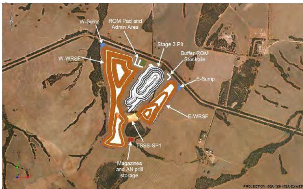
Figure 3-19: Pit and mining infrastructure - Stage 3 (AMC 2015)
