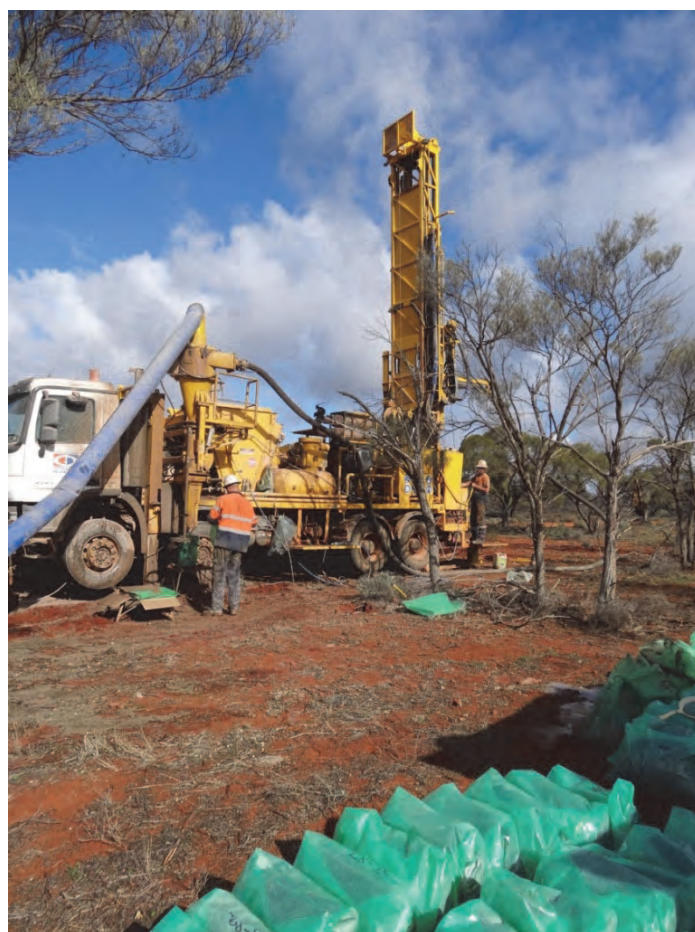
Figure 9: Drill-hole 13RSDRC01 targeting a marginal magnetic zone of intrusive complex
