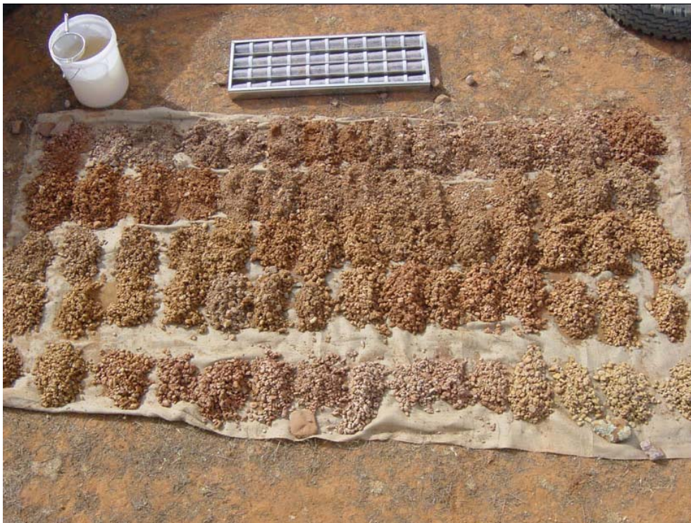
Photo 4 Portion of typical sample line and modified core tray containing 250ml samples jars
