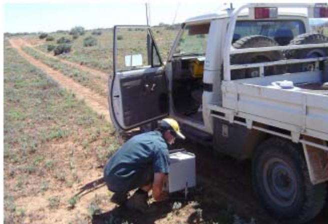
Photo 2 –Crew member Clinton Withish performing Gravity and GPS Acquisition.
