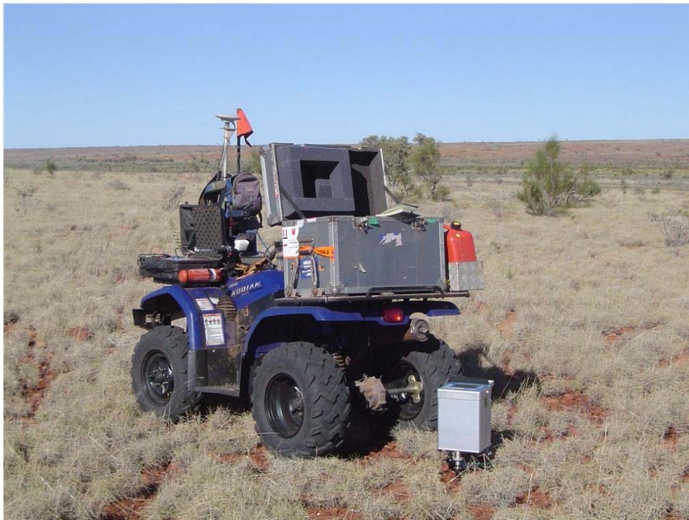
Photo 2: GPS-Gravity Acquisition using quadbike
